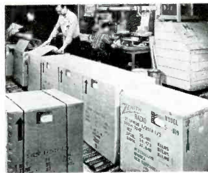
Sealing Zenith Radio export cartons with Tape-Strap. Operation is said to take one minute in comparison to four minutes required to seal and strap with metal.
