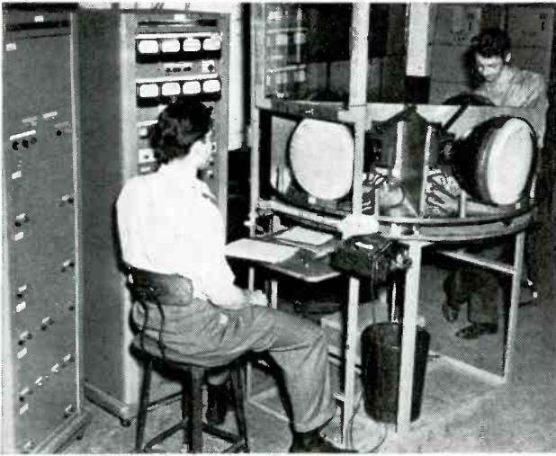
Turntable automatic picture-tube testing equipment.
