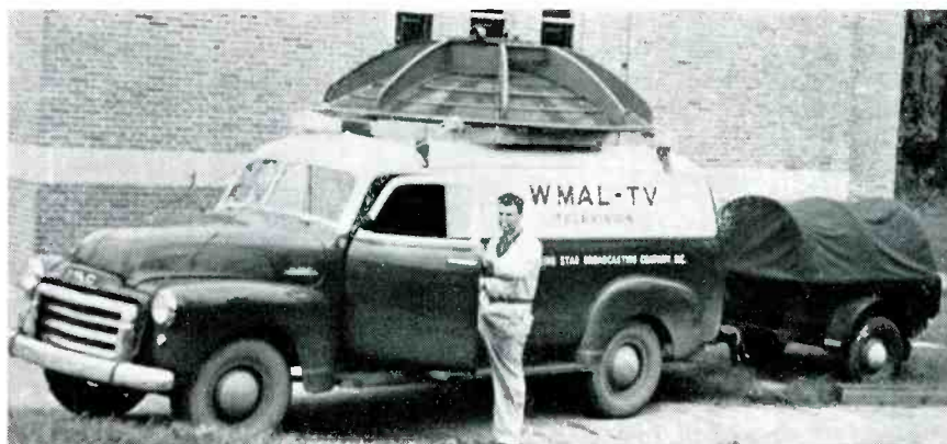
Figure 4 Relay truck loaded for special field test. Four, six and eight-foot reflectors are on roof rack. Equipment for the 2000 and 7000-mc system is in the truck, and a 110-volt gas-engine power plant is in trailer.
