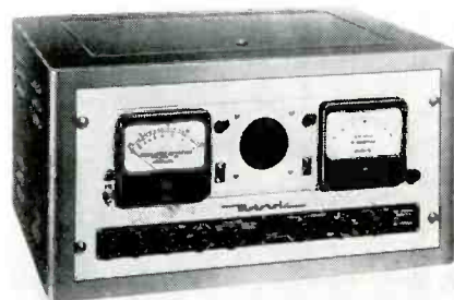
Motorola frequency deviation monitor
