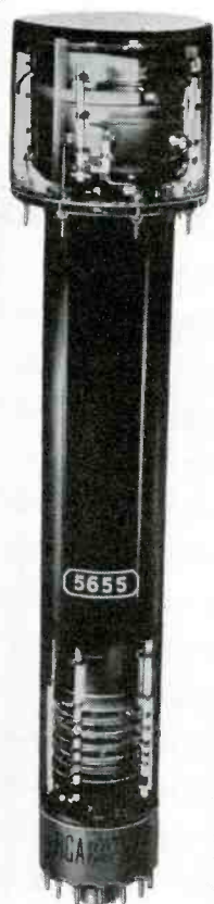
An image orthicon, type 5655. (Courtesy RCA)
