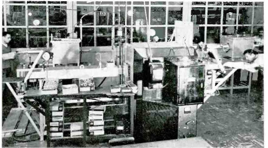
Specially-designed and constructed furnaces which are used for hydrogen-firing of all stainless-steel parts used in the electron guns.
