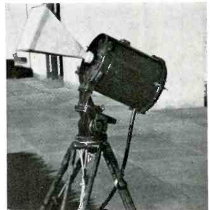
Figure 2 (left) Intermediate setup for two link relay of special telecast where a six-foot reflector, used with a 7000-mc receiver, served to pick up signals from a point of program origination 17 miles away, and a 2000-mc transmitter and four-foot reflector was used to direct signal to WMAL-TV 57 miles away. In this view appears a closeup of the special scaffolding and antennas used in setup.
