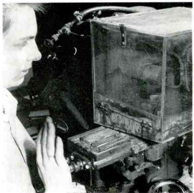
(Left and below) Sawing pellets from a thin slice of germanium from the ingot.
