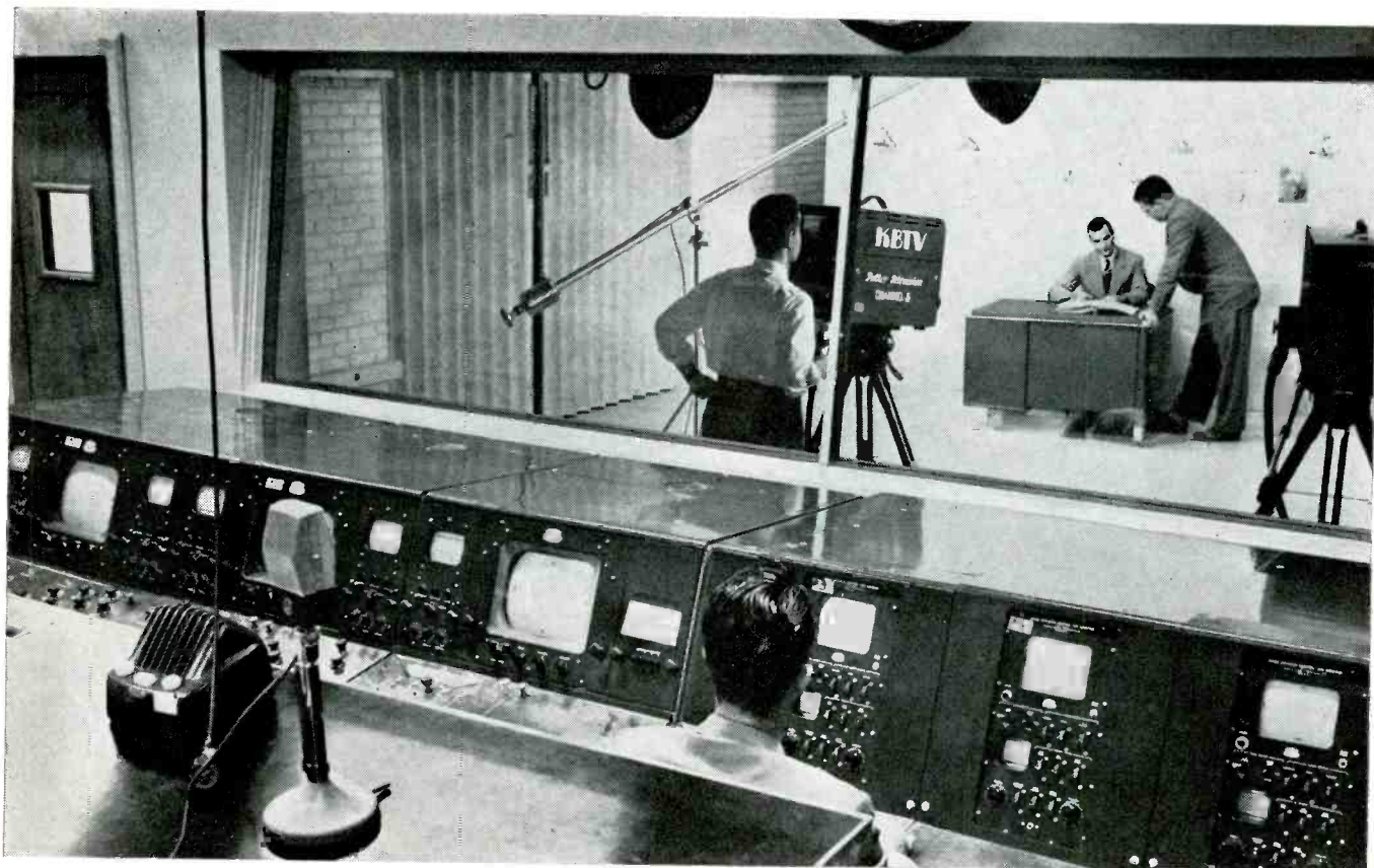
Looking in, from the director's table in the control room to the studio; at left, two film-shading generators and monitors, and at right, three camera-chain control units.
