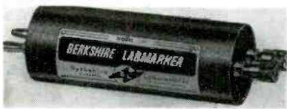
Wave-shaping unit developed to produce time marks for 'scope work.
