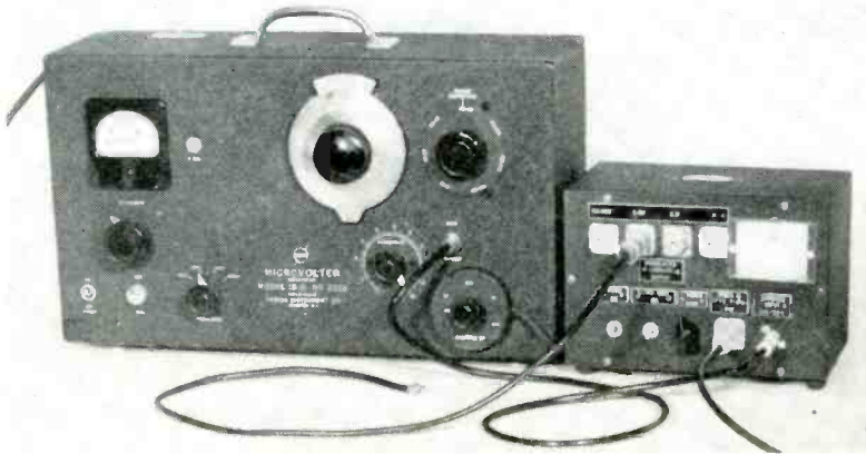
Figure 1 Setup of the rf signal generator developed at DuMont (right) connected to a standard vhf standard signal generator.
