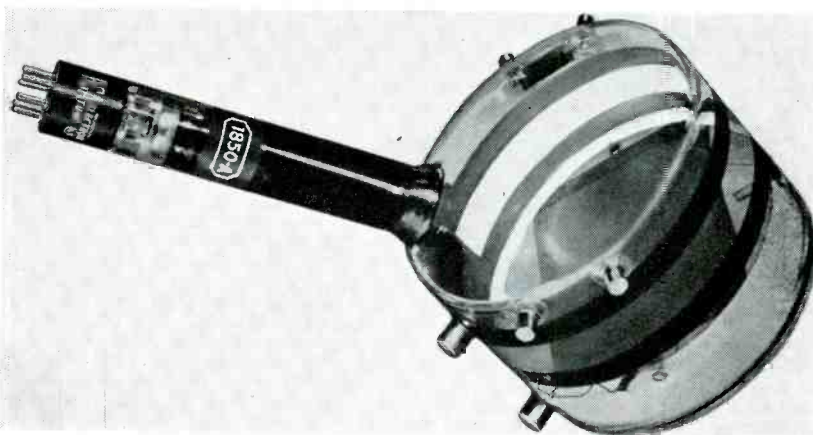
Figure 5 An early type of iconoscope; type 1850-A.
