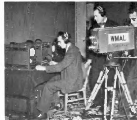
WMAL , Washington, D. C., picks up an indoor event with its new image-orthicon camera. Monitoring is done at the easy-to-carry, suitcase-type control units.
