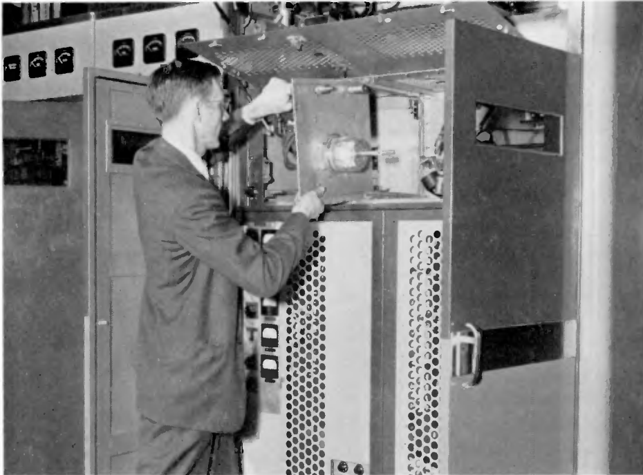
Engineer demonstrating ease of installing new power tube unit, 8D21, heart of RCA 5 KW transmitter. New transmitter is installed at WNBW, Washington, D.C., video station. Tube permits operation on all 13 tele channels.
