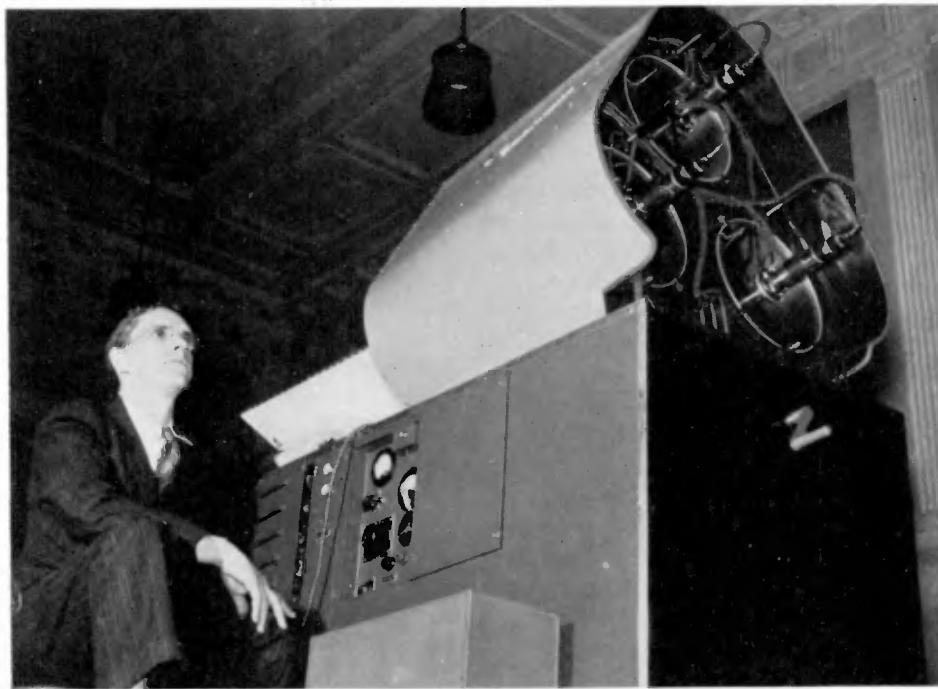
RCA's large-screen color television projector as demonstrated at Franklin Institute, Phila. Note three special kinescopes which receive and project green, blue and red picture signals. Operator can control and mix colors. Unit, still in process of development, projected pictures on a 7½' x 10' screen. Also used for B. & W.
