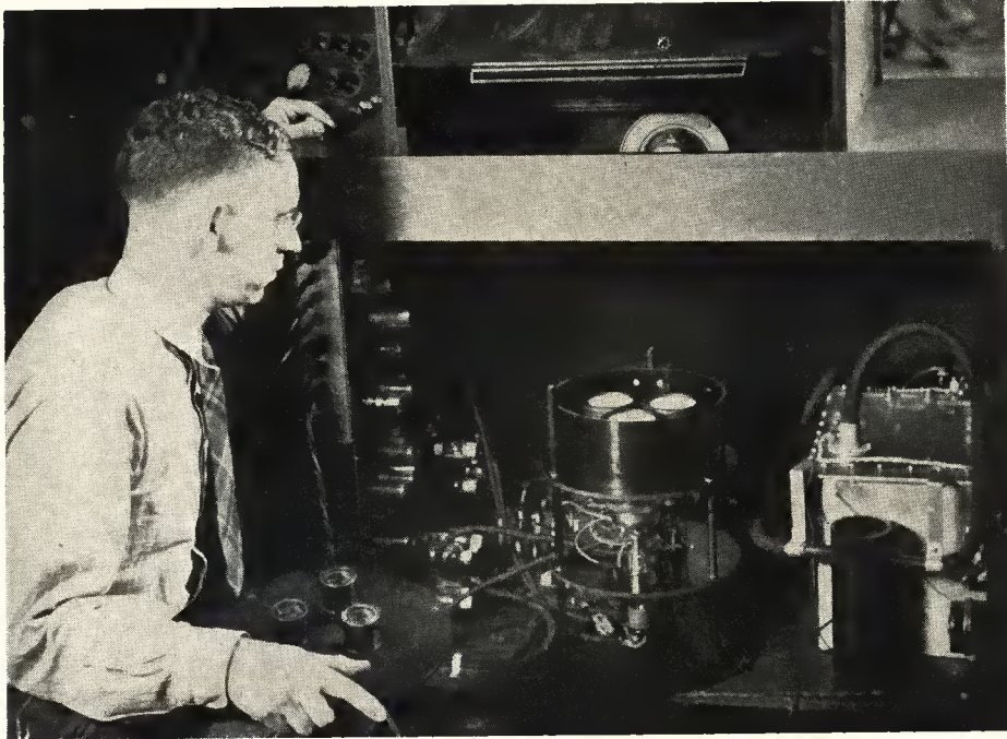
Chassis-view of RCA's all-electronic color tele receiver, showing "Trinoscope," three picture tubes (center). Engineer is holding projection lenses cover which fits over Trinoscope.
