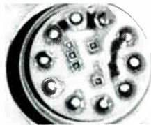
TO5 header showing cermet resistors and transistor dice.
