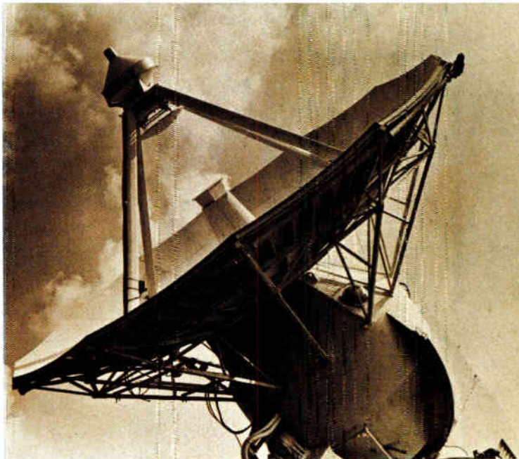
Antenna system, 30-ft. diameter, for Apollo Unified S-Band tracking/communication system built by Collins Radio for Nasa-Goddard.
