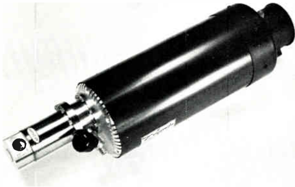
The "Cryomite" closed cycle cooler by Malaker. The mercury-doped germanium infrared detector is mounted behind the window at left.
