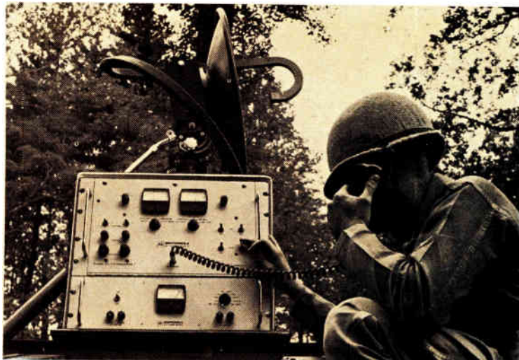
MP-7 portable microwave equipment can be placed into operation within minutes after being placed at a battle scene (Motorola).
