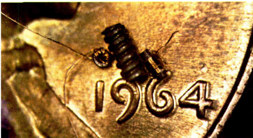
A toroid, slug, and transformer on a penny. Background is dark and aids in showing subtle color differences of the units.
