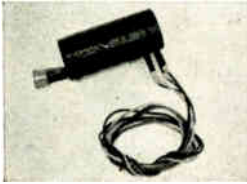
Connecting components of klystron leakage shield
