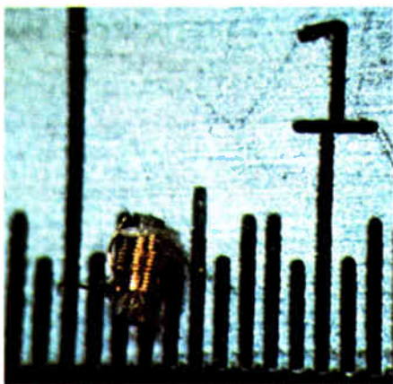
Tuneable transformer on a .01 inch per division rule. The background for the object tends to distract from the subject.
