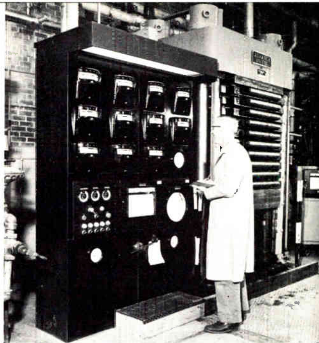
Heat and high pressure, applied to the piles, weld the laminations into a solid sheet and bond the metal foil to the base laminate.
