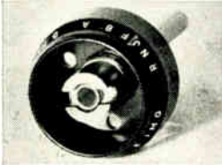
Assembling spindle tension cap for textile machine
