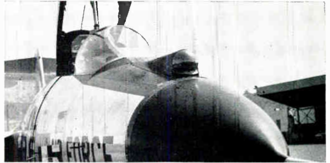
Interceptor IR installation
