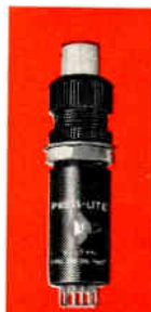
SW 616 alternate action SW 618 momentary contact 2 amp at 125 volts AC, 75% power factor 3/8" outside dia. Lamp Size - T 1 3/4
