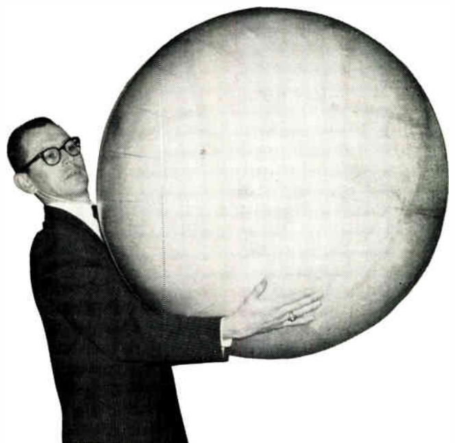
Fig. 6: Author R. L. Horst holds spherical lens assembled from cylindrical wedges. This lens was assembled dry; no adhesive was used on the interfaces. Weight of the lens is about 25 lbs.
