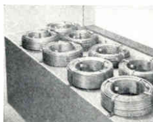
Designed for use in missile check-out equipment, this delay line consists of 285' of 3/8" diameter, 50 ohm Foamflex. The small, lightweight package is 16" in diameter by 6" high. Delay accuracy tests to \pm 1 nanosecond.
