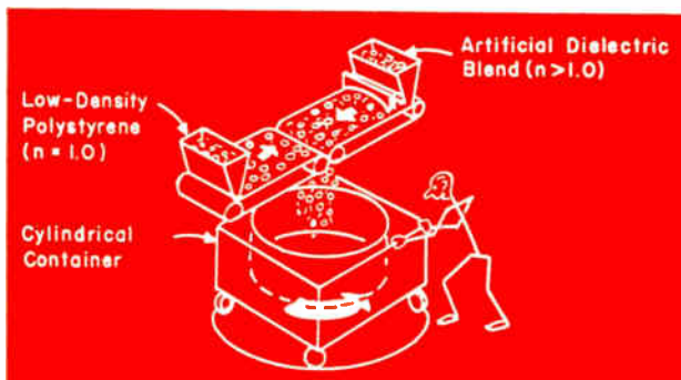
Fig. 4: Sketch shows variable-index cylindrical lens preparation.
