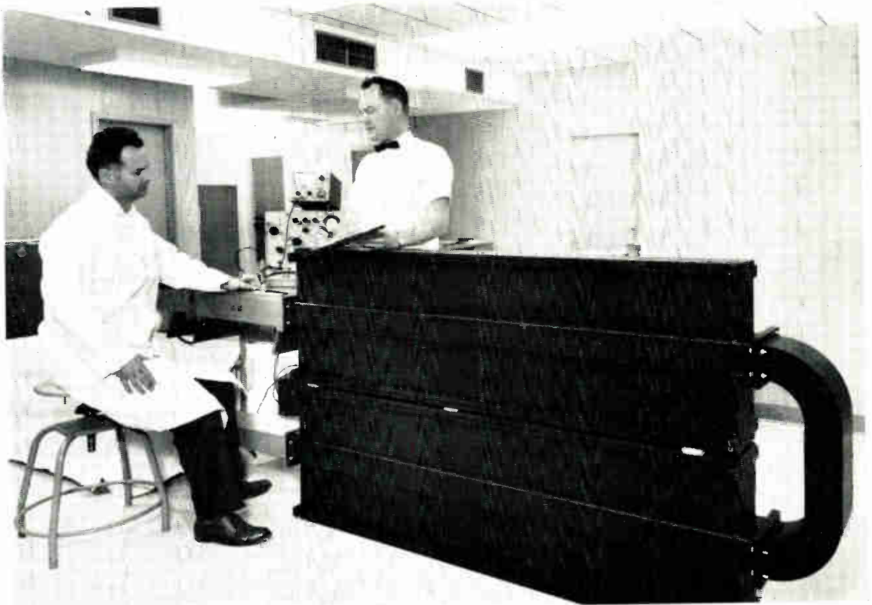
V. G. Price and a co-worker discuss results of tests which were conducted on this absorption type, highpower harmonic filter.
