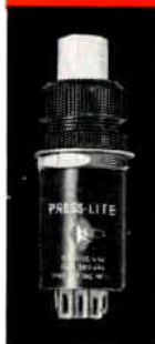
SW 617 alternate action SW 619 momentary contact 15 amp at 125 volts AC, 75% power factor 7-1/2 amp at 250 volts AC, 75% power factor 3/4" outside dia. Lamp Size - T 1 3/4
