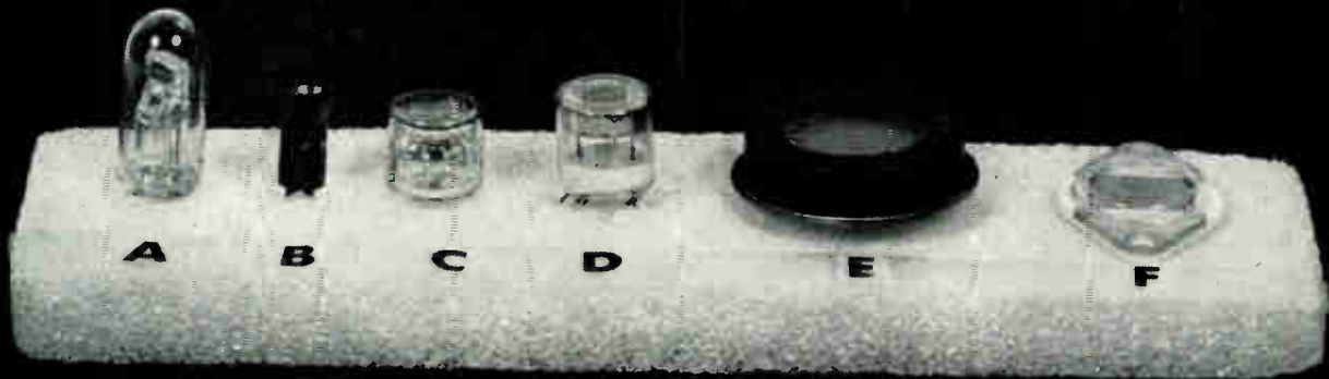
Fig. 2: Some available photoconductive devices: A is a single crystal cell; B is a small area sintered cell; C is a pressed-powder pellet; D, E, and F are all sintered powder on ceramic substrate with dissipation ratings of 0.5, 2, and 25 watts, respectively.
