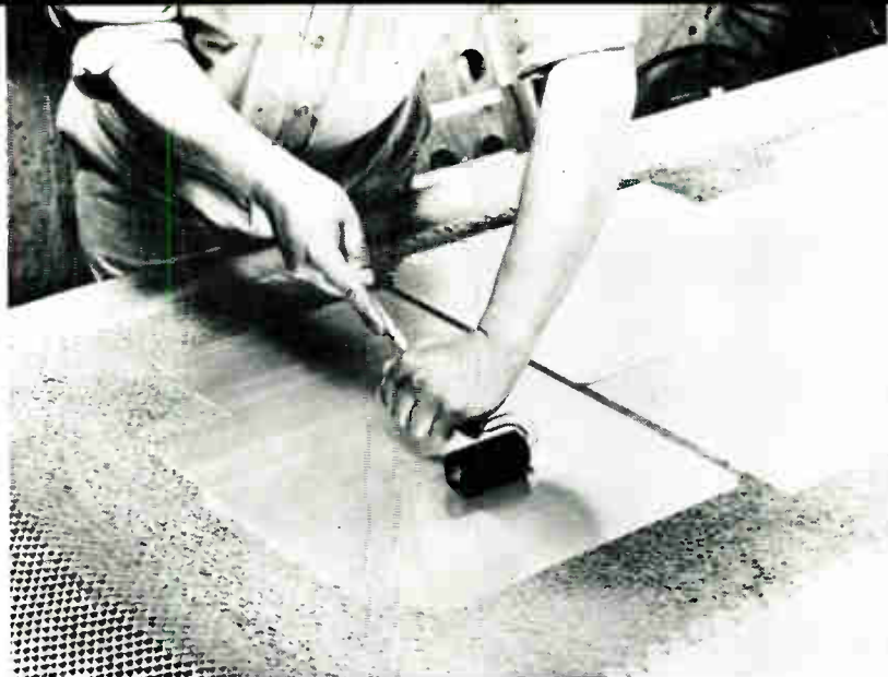
Above shows tape-bin panel fabrication using sprayable adhesive to bond sheet aluminum to a paper core. The panels can be handled as soon as assembled.
