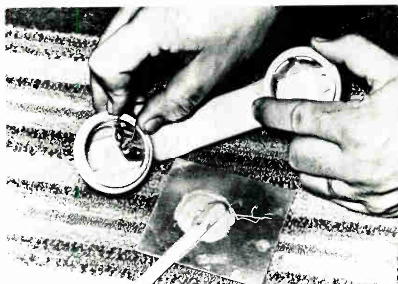
An example of bonding metal to plastic is seen above. Here, a two-part epoxy adhesive helps to position the on-off switch inside the shell of the phone.
