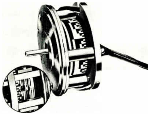
Above is a 128-count true binary encoder. Brushes and segments of this A-D encoder are magnified as brought out in the circle.
