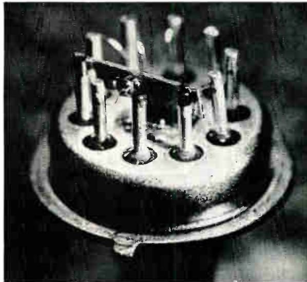
Hybrid microcircuit (above) on a transistor includes silicon epitaxial planar transistor bridge-mounted on pins and silicon chip with 5 thin-film resistors fixed to header (below).
