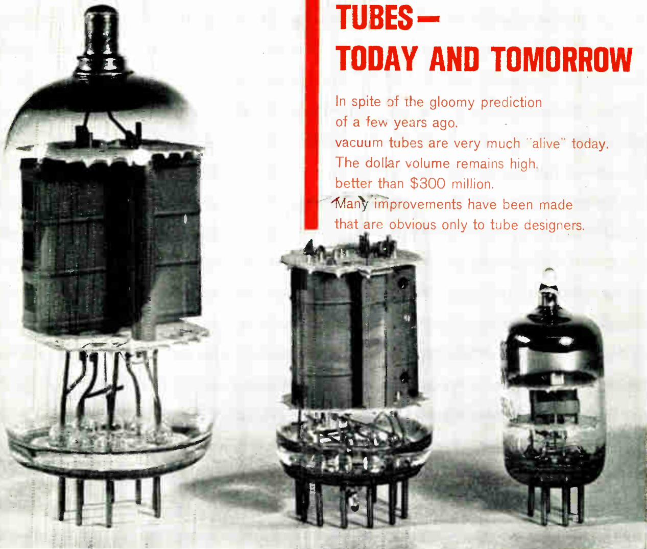
Fig. 1: The novar, compactron, and frame-grid constructions represent some of the newest types of tubes used today.
