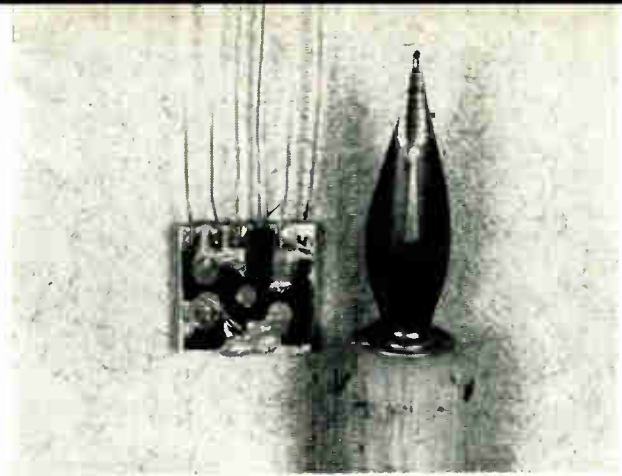
"The two major microelectronic circuits receiving attention from industry at this time are semiconductor-substrate circuits (below), passive-substrate, thin-film hybrids (above)."
