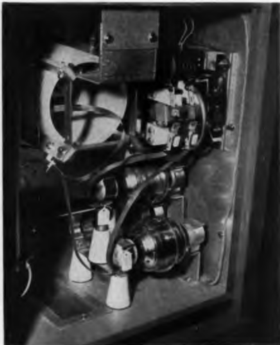
Gates Radio Company Broad-band Transmitter utilizing Jennings type M-1000 and M-750 Vacuum Fixed Capacitors.
