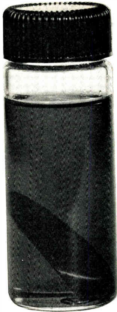
ORDINARY CHLORINATED SOLVENT under same conditions dissolves resin, damages metal.
