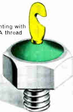
Type SB3A Screw mounting with \frac{1}{8} -32 UNEF-2A thread
