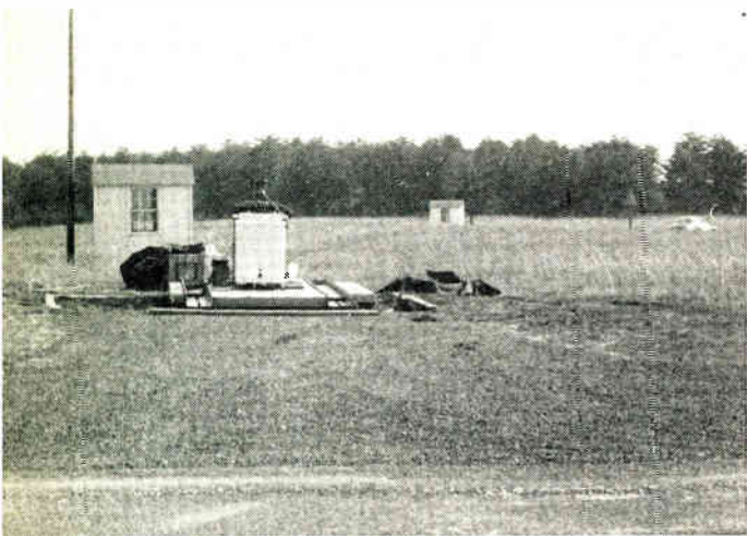
Fig. 10: View of diathermy test range at FCC Lab. shows equipment under test. Diathermy is mounted on a wooden turntable and measuring equipment is in wood shack. Lamps are dummy load.
