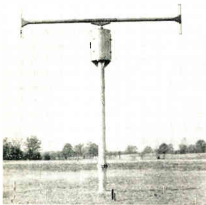
Fig. 7: A modern Adcock antenna used for long range direction finding from 2 to 30 mc.
