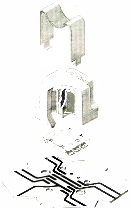
Exploded view of the Printact relay shows the basic elements. Printed wiring board is not an integral part of the relay.
