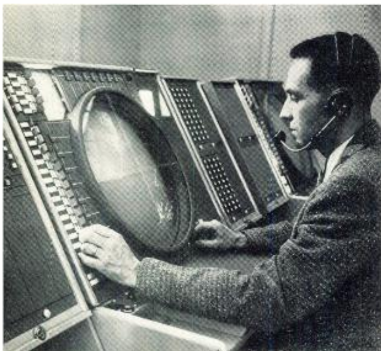
Picture of the air defense situation as picked up by SAGE network and analyzed by IBM computer, is flashed on this screen. With buttons and switches at sides, Air Force personnel make tactical decisions which are in turn carried out by the computer.
