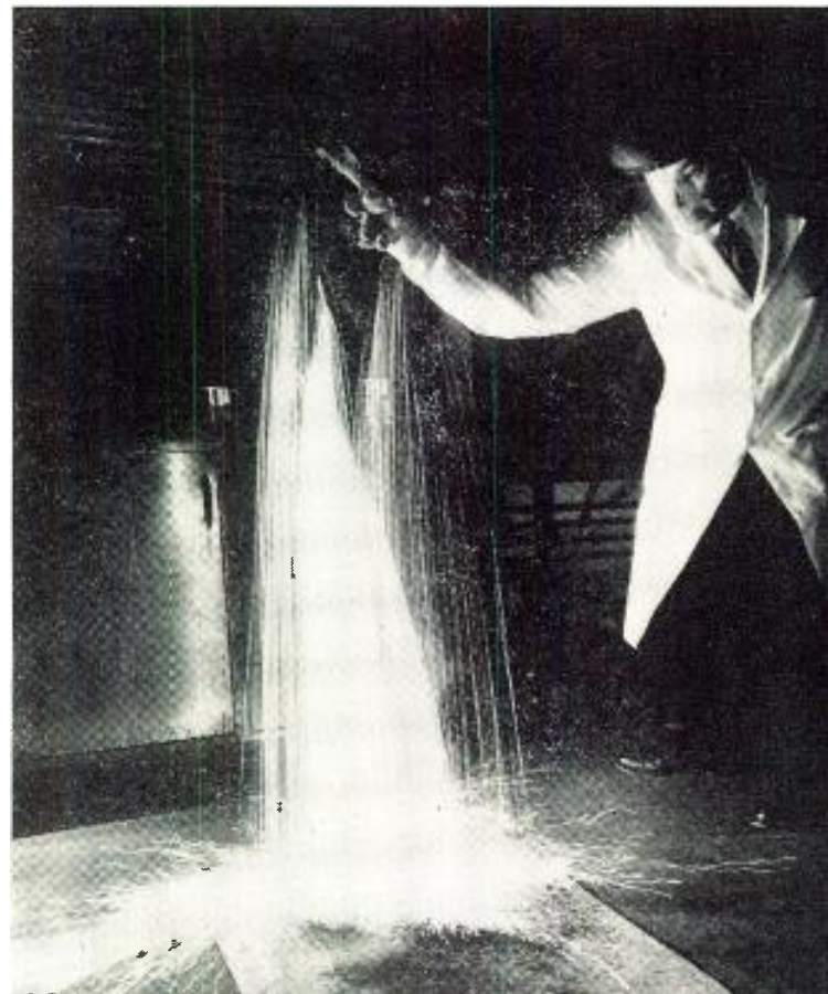
Highly purified manganese-bismuth powder bursts into a fiery cascade when exposed to air at Westinghouse Research Lab. Magnets made of the new material have more than 10 times the resistance of ordinary magnets to demagnetization.
