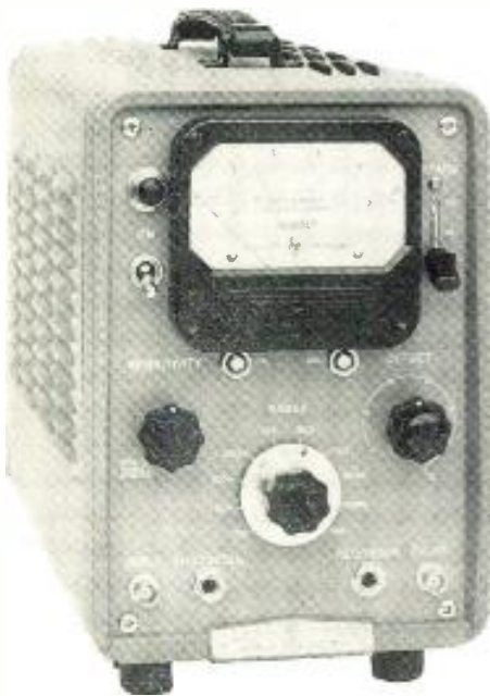
Fig. 1: Discriminator-output frequency meter measures 3 cps to 100 kc
