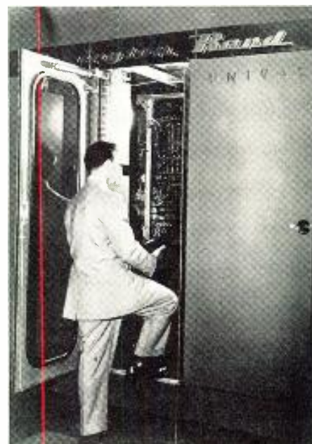
An 18,000-mile private wire system feeds all Sylvania data into this 10-ton central computer. Data correlation results previously requiring weeks can now be obtained in a matter of hours
