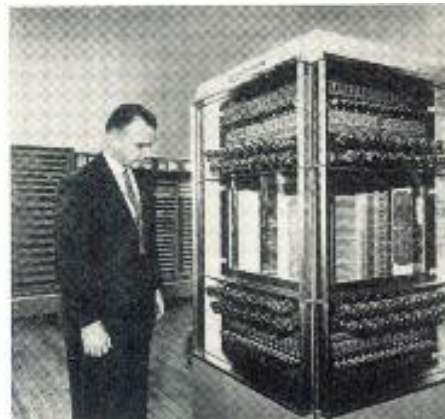
One of the Memory Array Frames which comprise the heart of the AN/FSQ-7 SAGE computer
