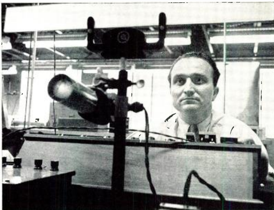
Scientist at control box of a Sanford-Bennett High-H-Permeameter measures hysteresis loop of Indox ceramic magnet.
