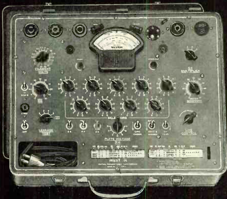
Weston Model 981 Proportional Mutual Conductance Tubechecker
