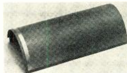
Fig. 2: Shield cloth, already formed here, is printed in a continuous strip
