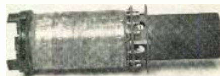
Fig. 5: Completed yoke consists of horizontal and vertical coils, and layers of shielding
