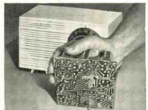
COMPACT, LOW COST RADIO. G-E Thru-Con Board permits compact chassis which slips into cabinet and plugs into speaker. Printed circuitry permits savings—cuts retail cost.
