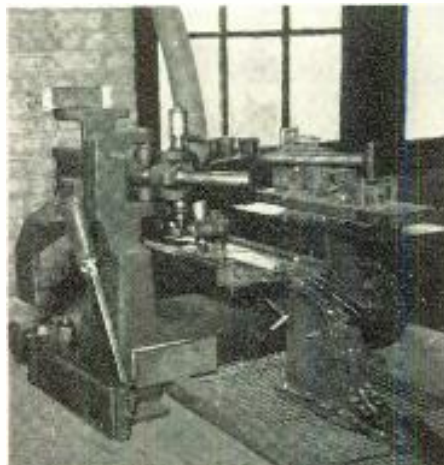
Fig. 5: Engraving machine modified to handle irregular-shaped components
