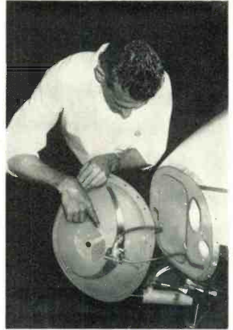
Bill Vogel, factory service mgr. at Lear Inc., points to Lear glide slope antenna, installed in nose section of Aero Commander. LF antenna is embedded in plastic. Perforations near apex of cone admit air for cabin ventilation.
