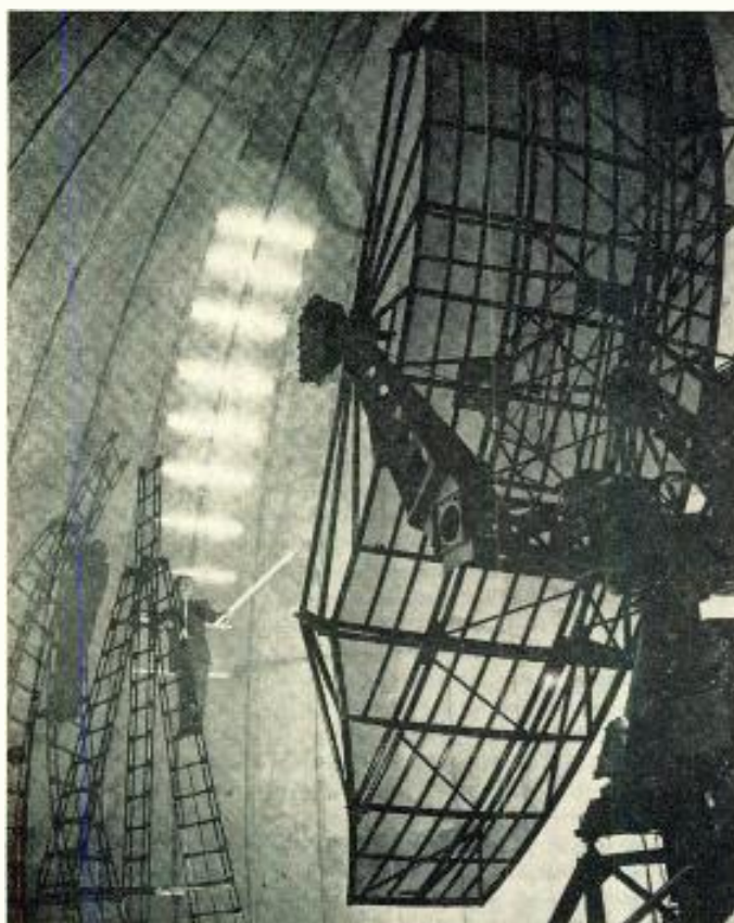
Fluorescent tubes are lit up by the multi-million watt radar beam from this Air Force FPS-6 height finder at GE. Engineer Z. Zenon, on the ladder, holds another lighted tube. Procedure is part of a study being made of radar beam effects.
