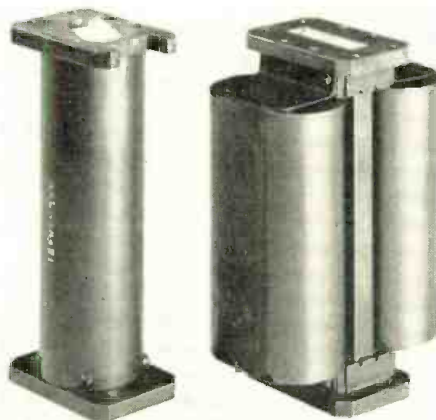
Fig. 5: Rotational type (l) and resonant-absorption type (r) ferrite isolators
