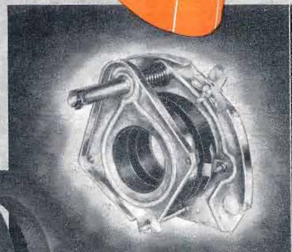
EXAMPLE OF A COMPACT TV FOCUSING DEVICE USING MAGNADUR RINGS
