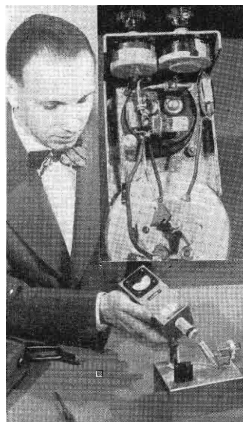
Clarence A. West, an RCA engineer, holds the transistorized grid-dip oscillator developed as a private project. Unit, shown in inset, measures 5 x 2 1/4 x 2 1/4 in., consumes only 25 mw
