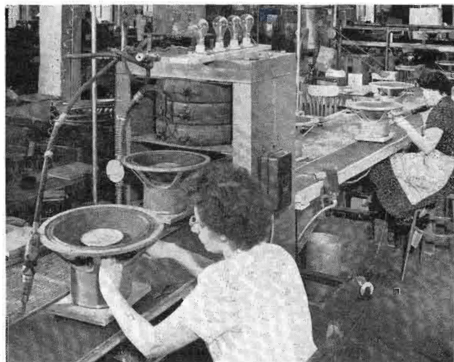
New 2.5-ton magnetizing unit goes into operation in Stromberg-Carlson's Sound Division plant, Rochester, N. Y. Photoelectrically controlled, unit consists of steel yoke supporting two pole-pieces each one foot in diameter. Each of the three coils on each pole-piece has 1450 turns of No. 12 cotton-enamel copper wire. (700 lbs. copper, total) In operation, 50 amps at 300 v. produces 10,000 gauss in air-gap. When magnetizing 10.5 lb. Alnico V polepiece in 15-in. speaker, the flux density rises to 14,000 gauss. Bulbs and heating coils are wired in parallel with magnet's coils to absorb power surges resulting from "on-off" operation.
