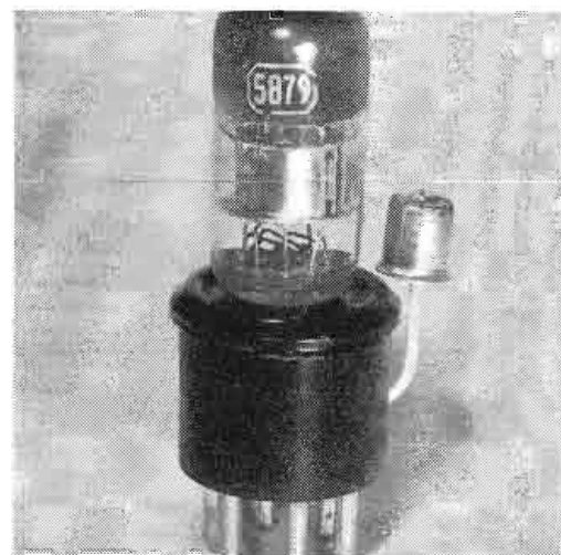
Appearance of 5879 tube mounted in adapter since the socket goes well into the base.
