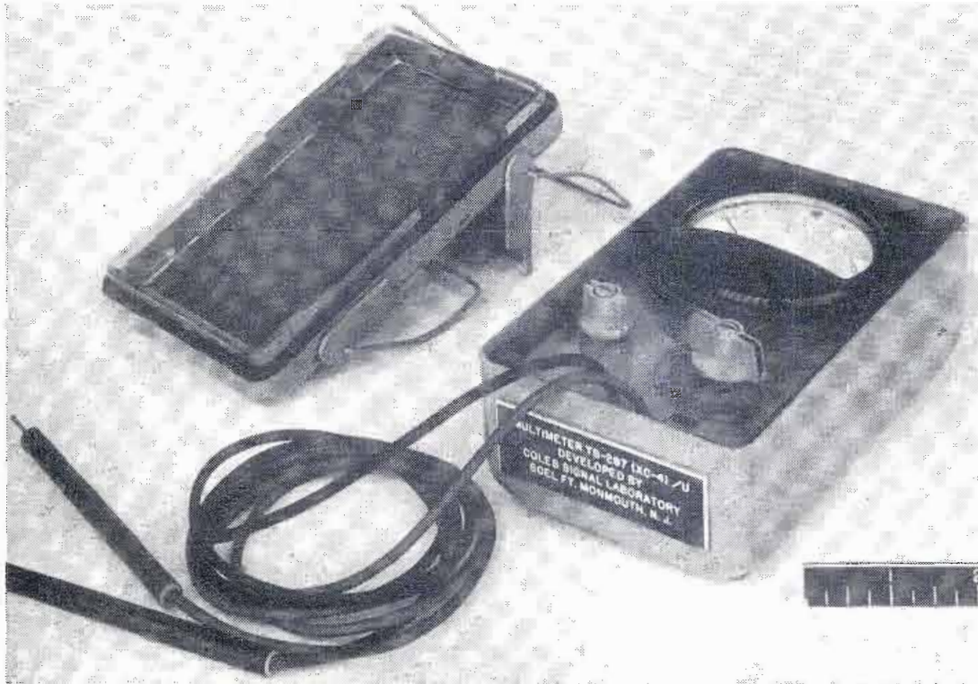
Fig. 1: Multimeter developed by Signal Corps Engineering Labs., with probes and cover removed
