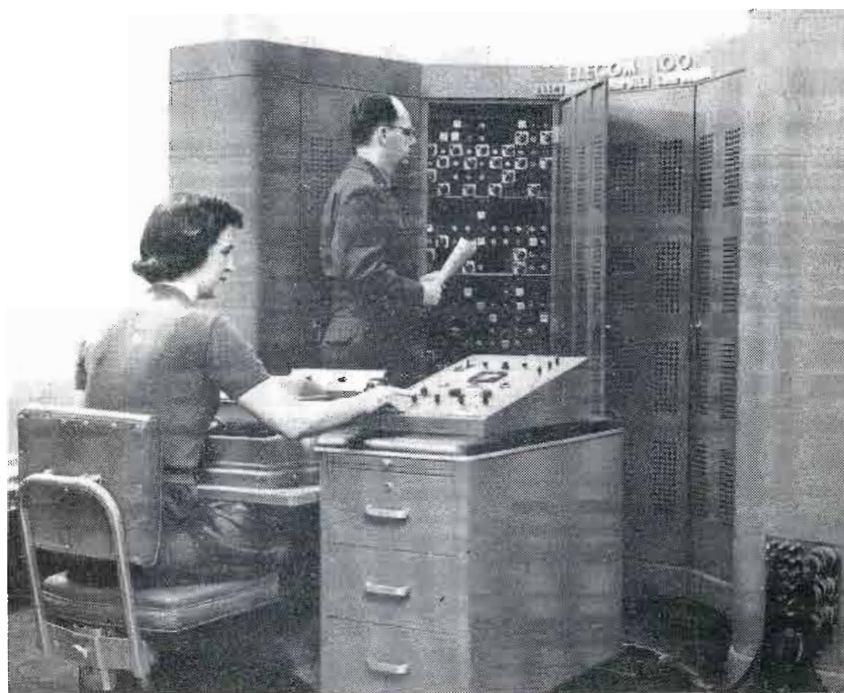
This first low-cost “robot brain” electronic computer available commercially for general use has been accepted by Army Ordnance officials at Aberdeen Proving Ground after it successfully completed sixty hours of grueling nonstop tests. Making errorless computations at the rate of 1700 a minute, this compact Underwood computer established a record unmatched in accuracy.
