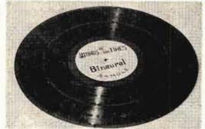
Fig. 6: Close-up of binaural recording shows the two bands of grooves
