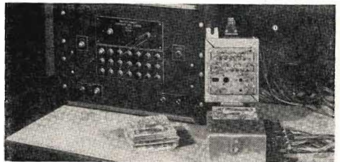
6 Finished and cut apart, the basic chassis is checked in two seconds by a stepped test set for leakage, shorts and opens
