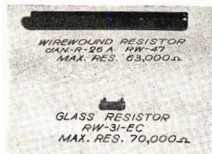
Fig. 4: Comparison of glass and wire-wound resistors shows small size of the glass type
