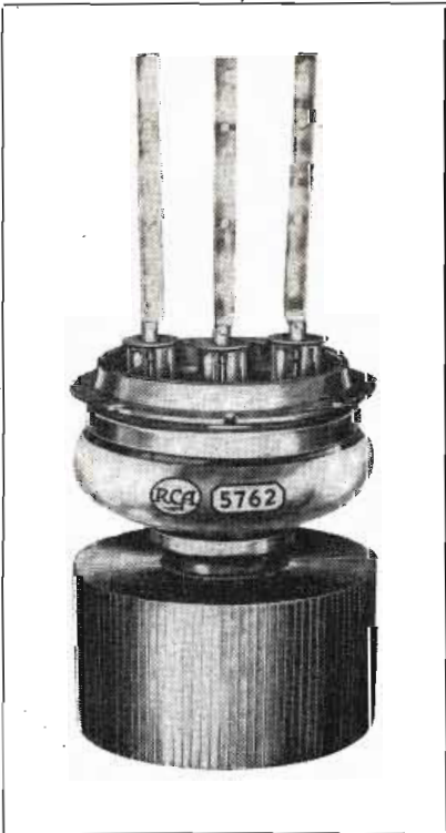
Fig. 4: RCA-5762 Power tube and cooler
