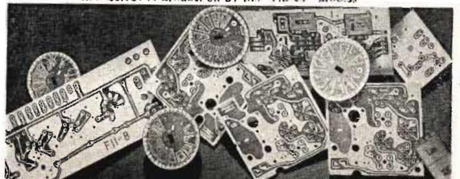
7 Wide variety of circuit shapes which readily lend themselves to production by the "Pla-cir" process
