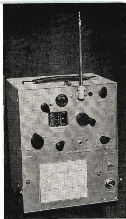
Fig. 3: Panel view of FM-3 VHF frequency meter
