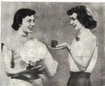
When solid aluminum silicate (right) is melted and subjected to a blast of air, fluffy cotton-like "Fiberfrax" fiber (left) is produced. In samples shown, weights are equivalent.
