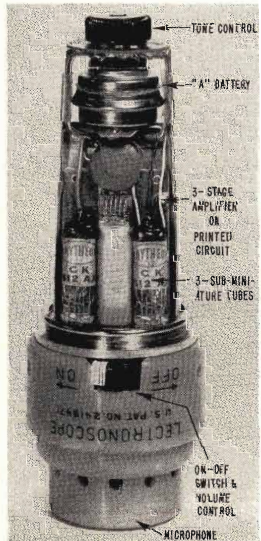
Construction details of medical stethoscope that uses three stage printed circuit audio amplifier and has self-contained batteries
