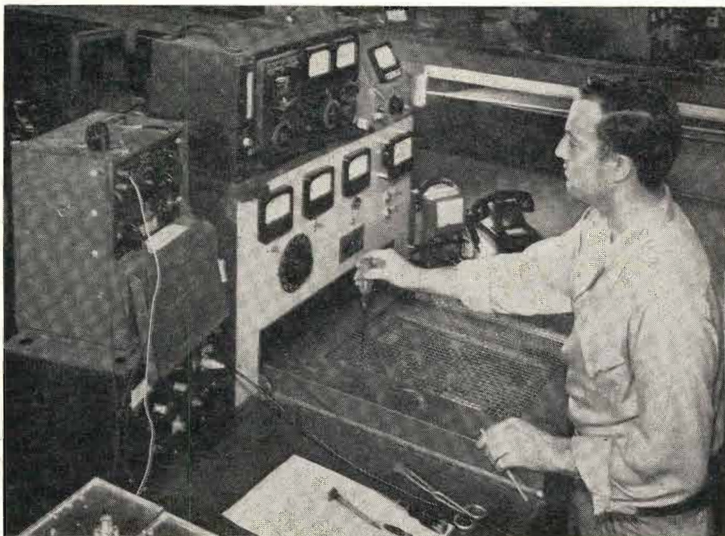
New type of shielded test bench on assembly lines at Motorola's new Chicago plant. Adjustments to equipment are made through screening which tips back to allow insertion or removal.
