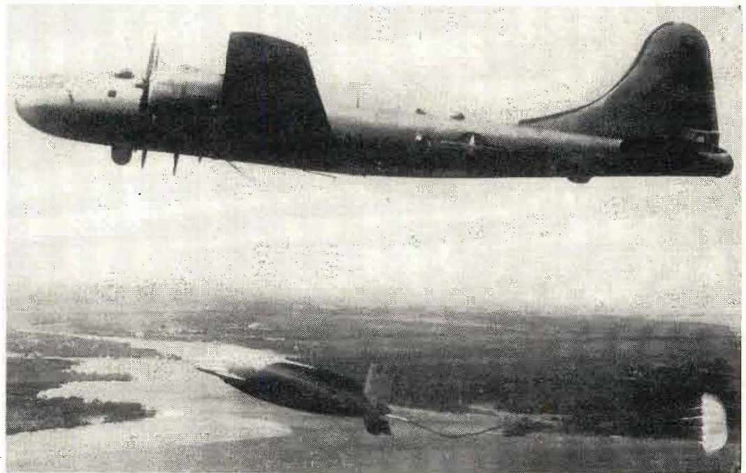
Lifeboat equipped with Westinghouse control system is parachuted to "survivors" in test run. Using one carrier with five different modulation frequencies, transmitter in airplane will direct boat
