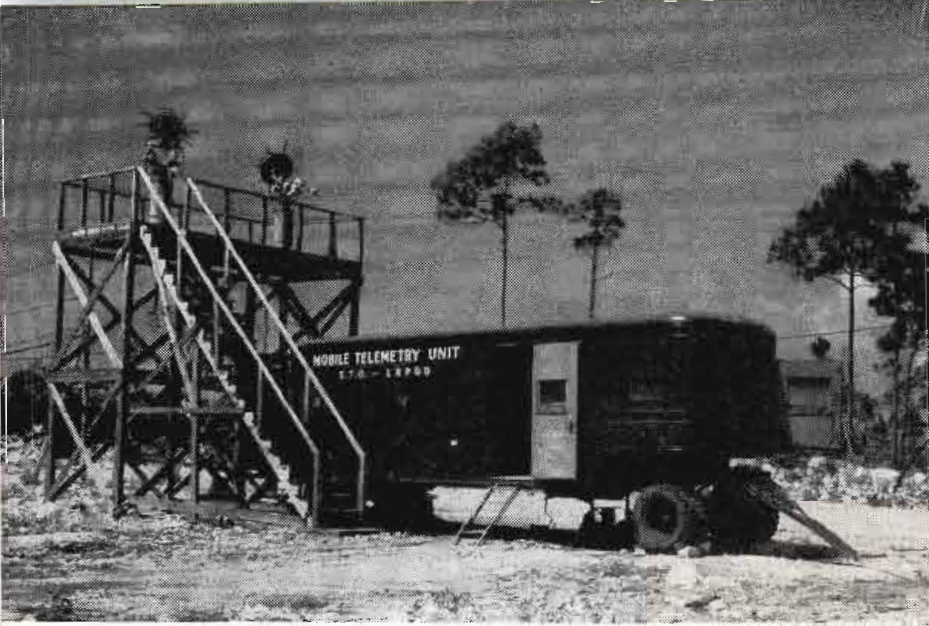
Fig. 1: Air Force telemetry facilities in the Bahamas record data from missiles in flight
