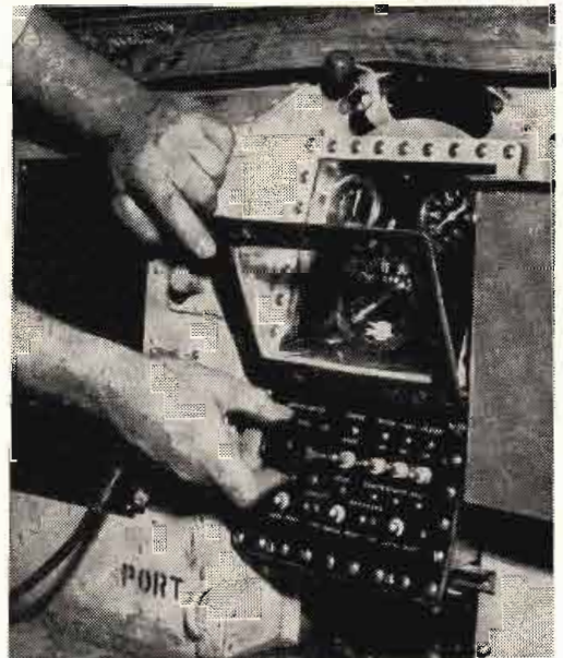
Push button controls enable weakened survivors to operate craft. Single master switch turns control over to aircraft radio operator
