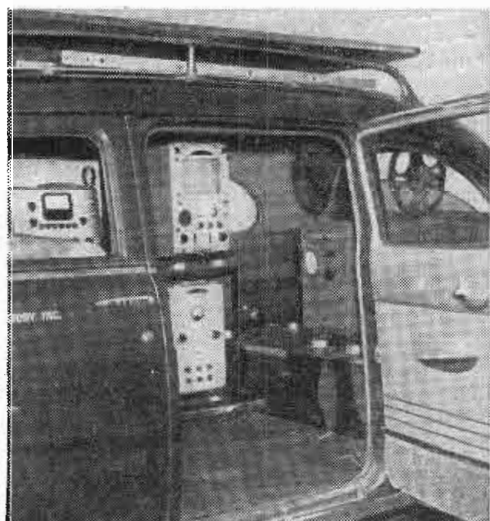
Included in cross-country demonstration unit is the GPL Utility Projector, with "3-2" intermittent which permits use with I.O. camera for film telecasting from remotes.
