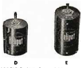
MODELS D AND E HELIPOTS Provide extreme accuracy of control and adjustment, with 9,000 and 14,400 degrees of shaft rotation. D—25 turns, 234" coil, 3-5/16" dia., 15 watts—resistances from 100 to 750,000 ohms. E—40 turns, 373" coil, 3-5/16" dia., 20 watts—resistances from 200 ohms to one megohm.
