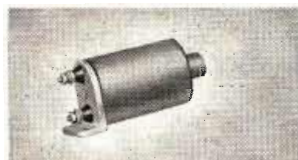
#1154 an intermittent service solenoid, 12v, D.C.—10.5 amps.—stroke 9/32", weight 13 oz.
