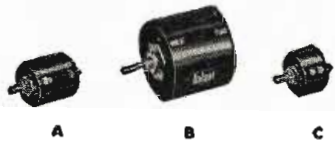
MODELS A, B, & C HELIPOTS A—10 turns, 46" coil, 1-13/16" dia., 5 watts—resistances from 10 to 300,000 ohms. B—15 turns, 140" coil, 3-5/16" dia., 10 watts—resistances from 50 to 500,000 ohms. C—3 turns, 13-1/2" coil, 1-13/16" dia., 3 watts—resistances from 5 to 50,000 ohms.
