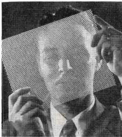
Section of a glassprinted circuit formed by ultra-violet photography and hydrofluoric acid etching
