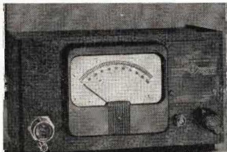
Fig. 17-18: (Left & Center) Panel and bottom views of logarithmic amplifier. Meter deflection is detectable for 25 microvolts input, full scale for 5-50 volts. Chassis is shock mounted to minimize microphonics. Fig. 19: (Right) 400 and 1000 cps filter for use in amplifier input. Inductance is wound on toroidal molybdenum-permalloy dust core and is shielded with can to minimize pickup
