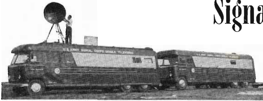
New tandem transmitting station. Lead vehicle houses complete camera pick-up and transmitting equipment and is interconnected to power supply coach by 4-wire cable
