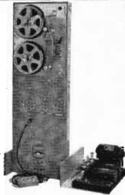
Multi-channel recorder for seismograph data recording in the field with remote control. Custom construction by AMPEX.
