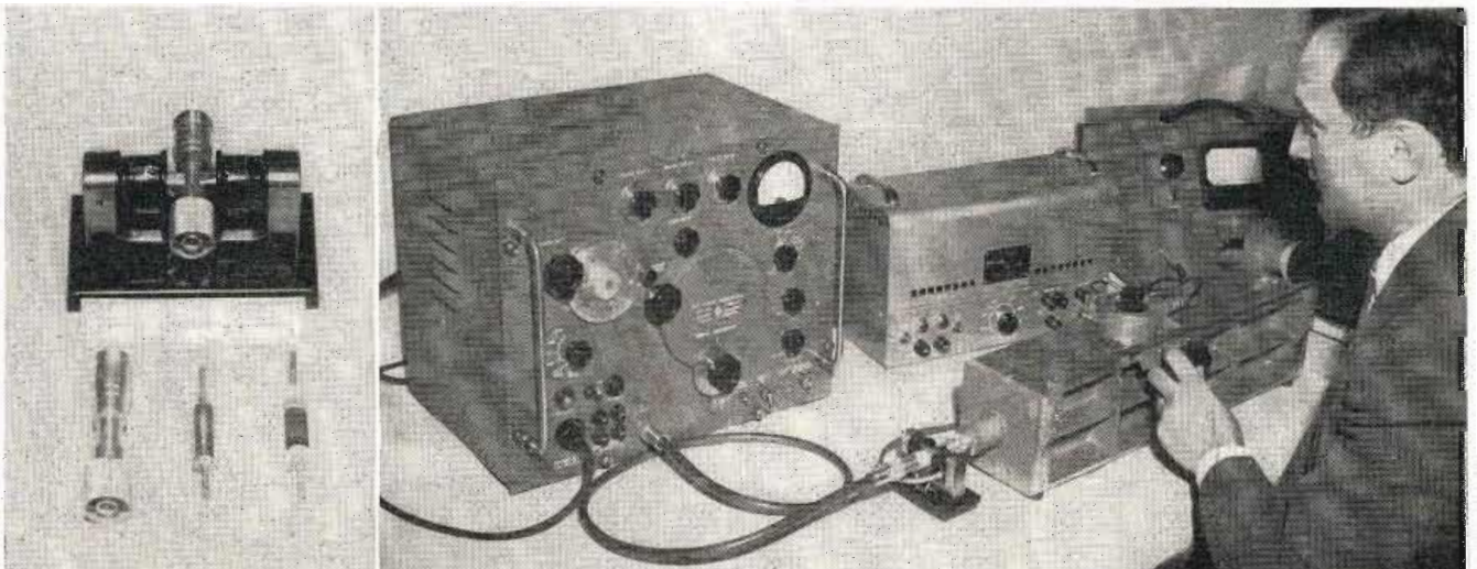
Fig. 2: (Right) Device inserted into a coaxial transmission line test set-up. UHF oscillator at left supplies r-f energy, regulated power supply, rear-center, provides dc to control attenuator, latter feeds standing wave meter, center-foreground
