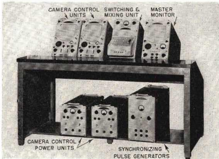
Fig. 1: Equipment units required in the control of two image orthicon chains. Compactness, stressed in design, makes each chain portable and enables quick field setups
