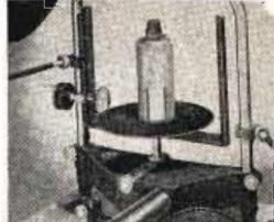
Rotating table, horizontally mounted, with friction drive
