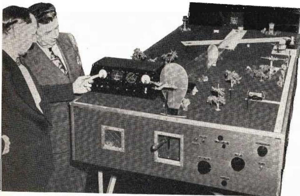
Fig. 4: Full operational model designed by the author (left) to demonstrate all the facilities mentioned in this article. ASR and PAR screens, rear, operate in phase with scanning radar antennae, and neon bulbs with RC network simulate radar blips. Every phase of approach control is authentically and visually illustrated by use of standard cockpit instruments. Unit is ideal for aviation radio aids instruction
