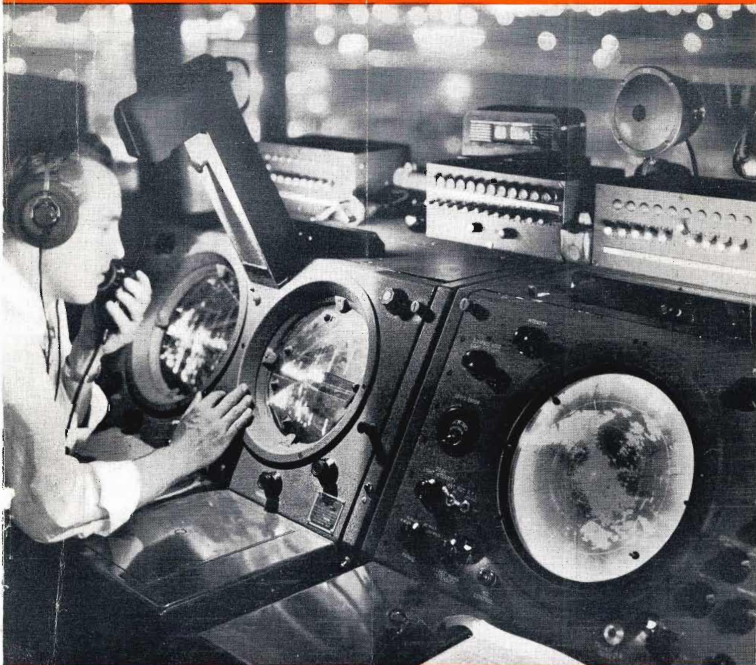
Ground Control Approach and Area Surveillance Radar at Los Angeles Airport, California
