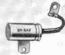
Aerovox Type 89ZAY using a metallized-paper capacitor and mounting inside voltage regulator case to work in conjunction with IN-127.
