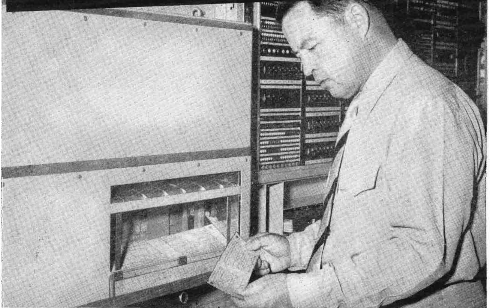
Studying punched card record of dial system operation. Each card (top) can report 1080 items
