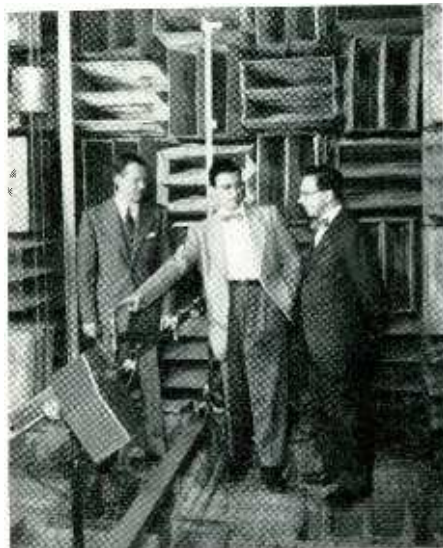
Interior of the new test chamber at M.I.T. Dr. J. J. Baruch, designer of the electronic components points to the traveling microphone while Dr. R. H. Belt (left) and Dr. I. L. Beranek (right), director and technical director of the laboratory respectively, view the equipment.
