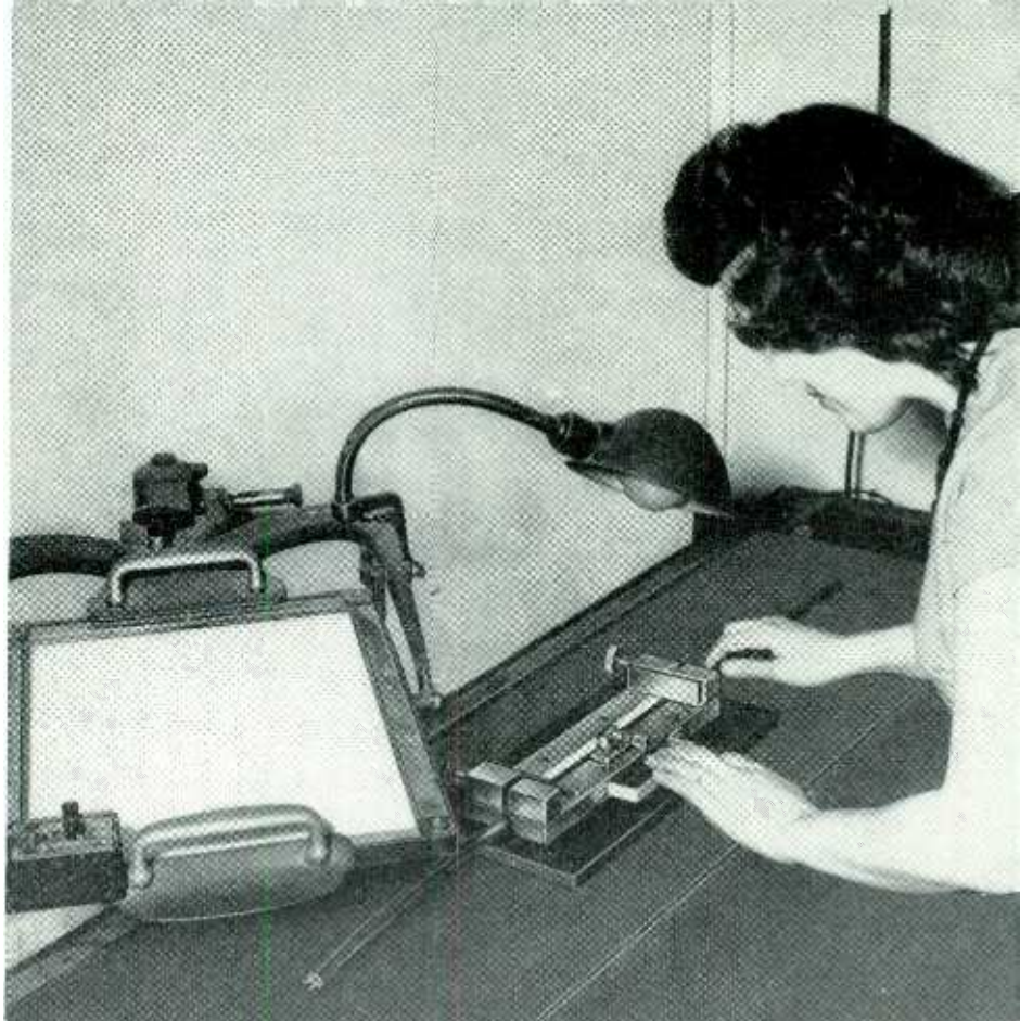
Fig. 1: Fluoroscopic coaxial cable eccentricity jig requires little training to operate
