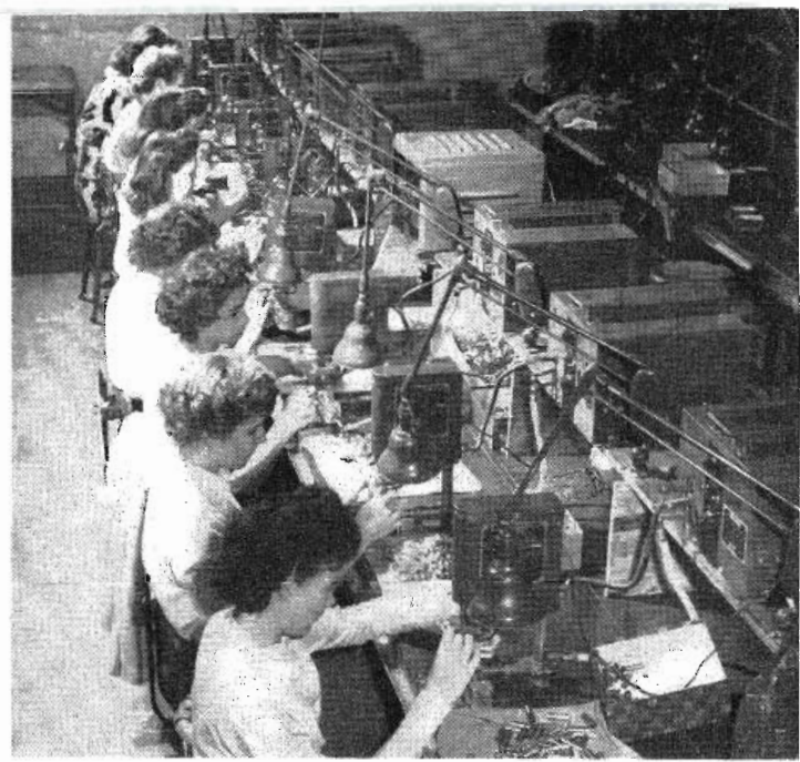
↑ View of operating stations in welding department where tiny supports and grid connectors are welded onto grid and anode assemblies. Supports on grids must be accurate to within 1°. All jigs and fixtures employed are manufactured in the plant
