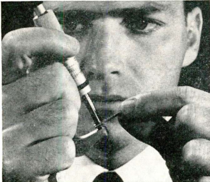
Trimpot reliability starts at the beginning. Here an incoming lot of potentiometer lead screws undergoes a dimensional check.
