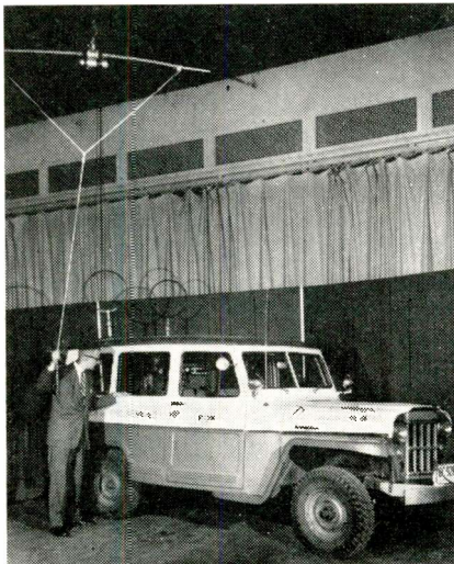
The specially-equipped vehicle measures high tension power line stress with the power-on by utilizing telemetering units.
