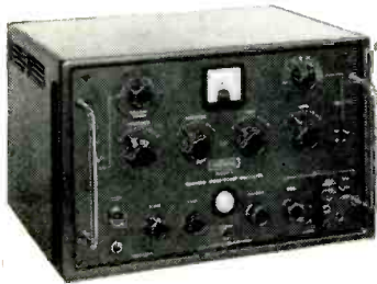
D-890-A (with crystal check) Frequency: 1c/s to 111.1kc/s Accuracy (max.): 0.05%; 0.005% at spot frequencies Output (max.): 126v into 8k ohms or 24v into 600 ohms
