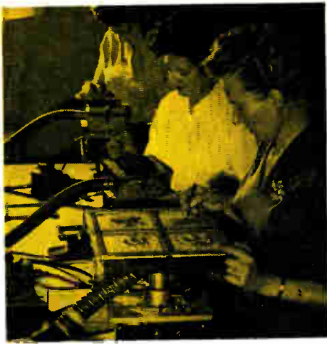
Pneumatic core positioner lines up ferrite memory cores so that girls can wire them
