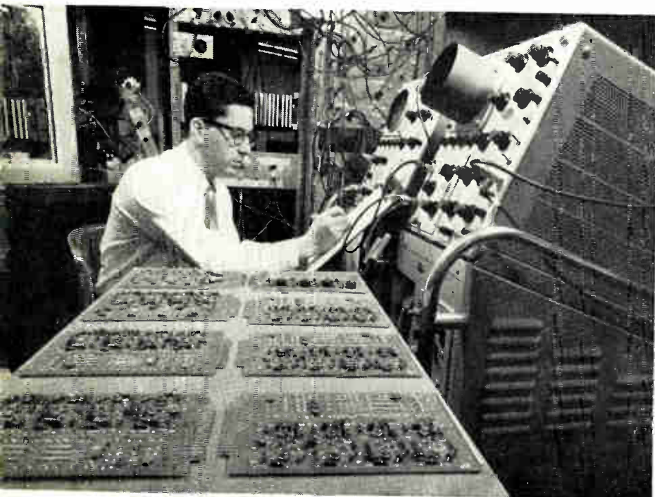
(l) Performance of new buffer memory is checked on oscilloscope at Applied Logics Division. (r) Frank Lewis checks new buffer memory designed for Kineplex transmission system
