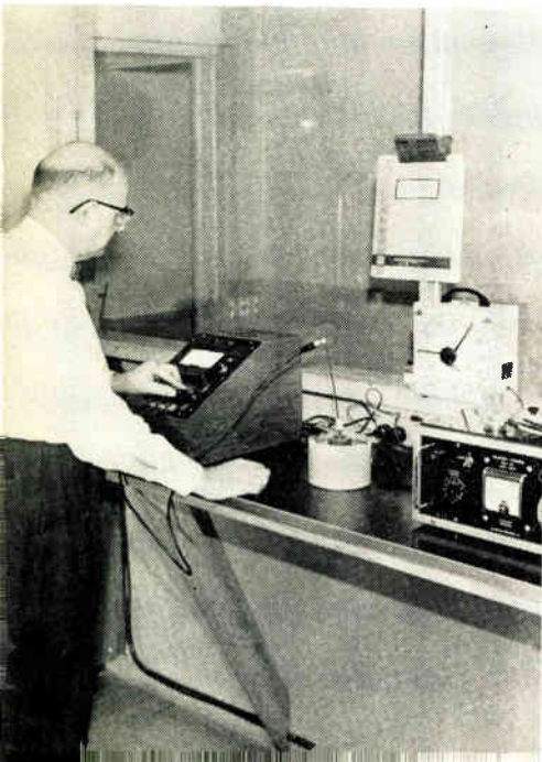
Hard coating of aluminum potentiometer mandrels increases life. Here a mandrel is checked for megohm resistance under mercury.
