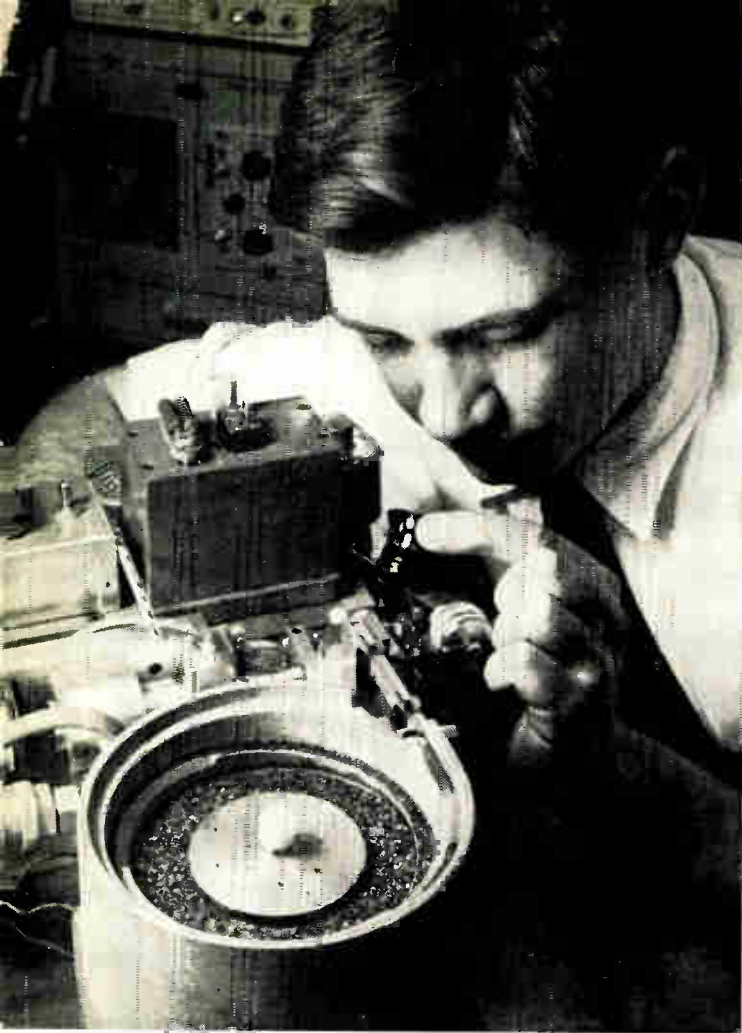
(Above) High-speed core handler that picks up and positions 12 cores per second is demonstrated by inventor, V. Goldswaithe
