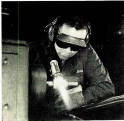
The plasma jet deposits tungsten in a plastic state on this spinning mandrel
