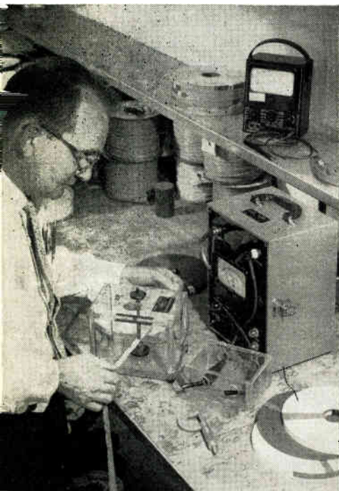
Fig. 7 (right): Cabler used to twist several single conductors into a multi-conductor.
