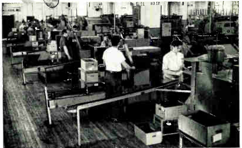
AUTOMATIC COLOR CODING MACHINES apply color bands and oven-bake the enamel at high temperatures to assure that the color coding will withstand the maximum operating temperatures of 150°C and all types of cleaning solvents.
