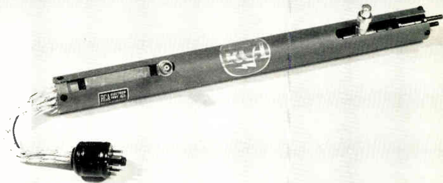
Fig. 2: The Estiatron traveling wave tube is electrostatically focused
