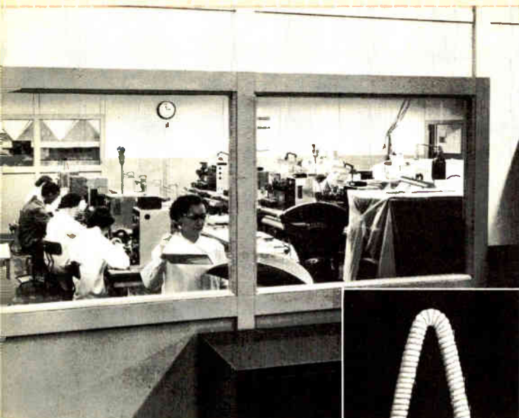
SYLVANIA'S ORIGINAL folded coil heater design is processed in this ultra-clean room to prevent contamination
