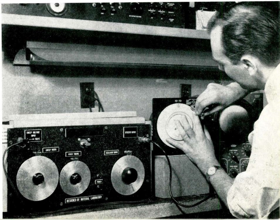
Main tuning dial of the Spurious Response Tester being aligned with the aid of a screwdriver.
