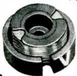
Bobbin, wound with specified number of turns of wire for desired inductance, placed in pot core.
