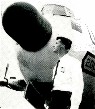
The beam from the radar set in the Douglas C-133A Cargomaster is detected by a new device worn by its designer, P. C. Barnes of Douglas. The alarm warns ground personnel to avoid high intensity radar beams.
