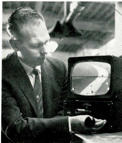
Kaiser Electronic Contact Analog Display System is demonstrated by its inventor, Geo. H. Balding. Kaiser was awarded a prime contract for the unit which provides the aircraft pilot with an analog of outside conditions.
