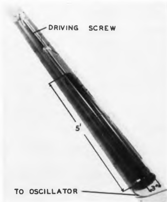
Fig. 1: The central conductor of this measuring line is supported by a metal disc at one end and the capacitance to be measured at the other.
