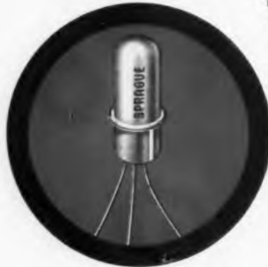
2N346/SB103 for High Frequency Oscillators
