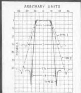
TYPICAL RESPONSE CURVES INDICATING THE VARIOUS SHAPE FACTORS AVAILABLE IN STANDARDIZED BURNELL CRYSTAL FILTERS
