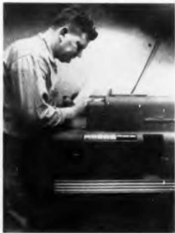
▲ Prepared beforehand, IBM cards are available for nearly every slab and strip size, and for each grade of steel.
