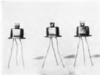
Fig. 2: Encased, Tecnetron looks like a transistor; characteristics, however, are more like those of a pentode tube.
