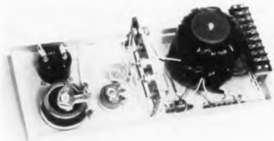
Fig. 5: Magnetic amplifier constant current power supplies reduced problems encountered in using electro-magnetically focused klystrons.
