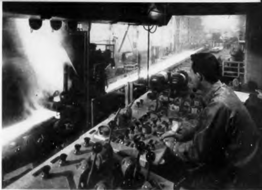
▲ In the Aliquippa Works of the Jones and Laughlin Steel Corp., a single IBM card controls all necessary variables in rolling a steel slab or strip. The Westinghouse automatic control system gives uniform production at the highest possible rate.
