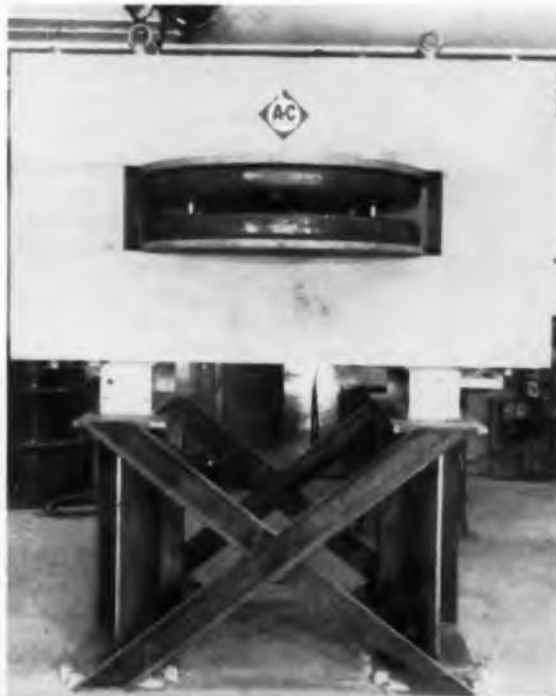
Fig. 1: Tests were run at fields as high as 10 kilogauss with this giant electromagnet. Semiconductors proved superior to tubes.
