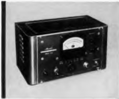
Micralino® 123B Wattmeter Bridge. Measures average power to accuracy of 3%. Self-balancing and direct-reading, bridge operates with Microline barretter or thermistor mounts. Frequency coverage depends on mount used.
