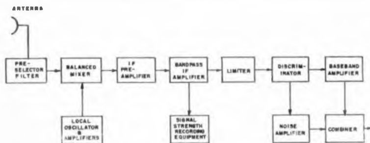
Fig. 7: An AGC controlled i-f metering circuit in the FM receiver measures field strength.
