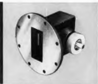
New Microline Barretter Mounts. For peak or average power measurements, these mounts are fixed-tuned and broad-banded to cover complete frequency range of their waveguide with high internal efficiency. Designed with low shunt capacity especially for peak power measurements with Microline 630 Meter. Barretters can be replaced by user. Three mounts cover all frequencies from 2.5 to 12.4 kmc.
