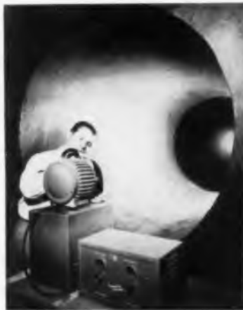
This subterranean 150-ft. tunnel beneath Federal Telecommunications' Labs' new R&D complex in San Fernando, Calif. is the latest advance in IR measurement facilities. Equipment can be run without interruption.
