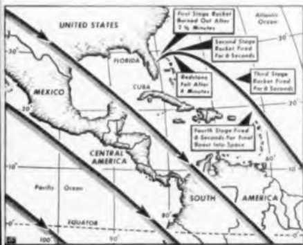
Explorer orbit is at 34° to the equator
