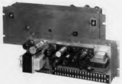
Ultra linear monitoring amplifier, all regulated power supply and speaker/warning light relays may be rack or desk mounted.
