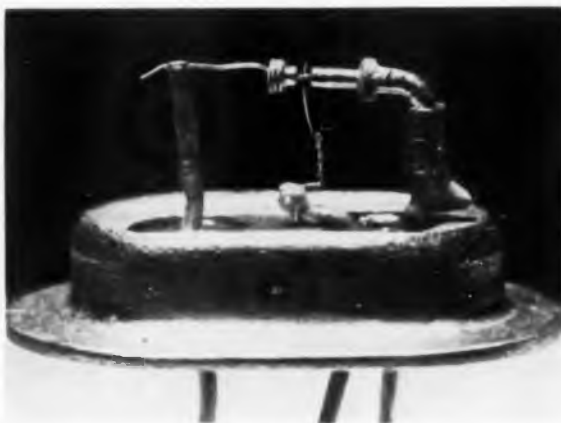
Fig. 1: The Tecnetron is made of a small germanium cylinder, 2 mm long, 5 mm in diameter, with a groove which acts like a tube grid.
