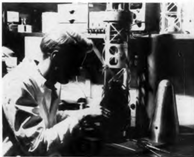
Satellite instruments are placed in "lattice sleeve" at Cal Tech's Jet Propulsion Laboratory
