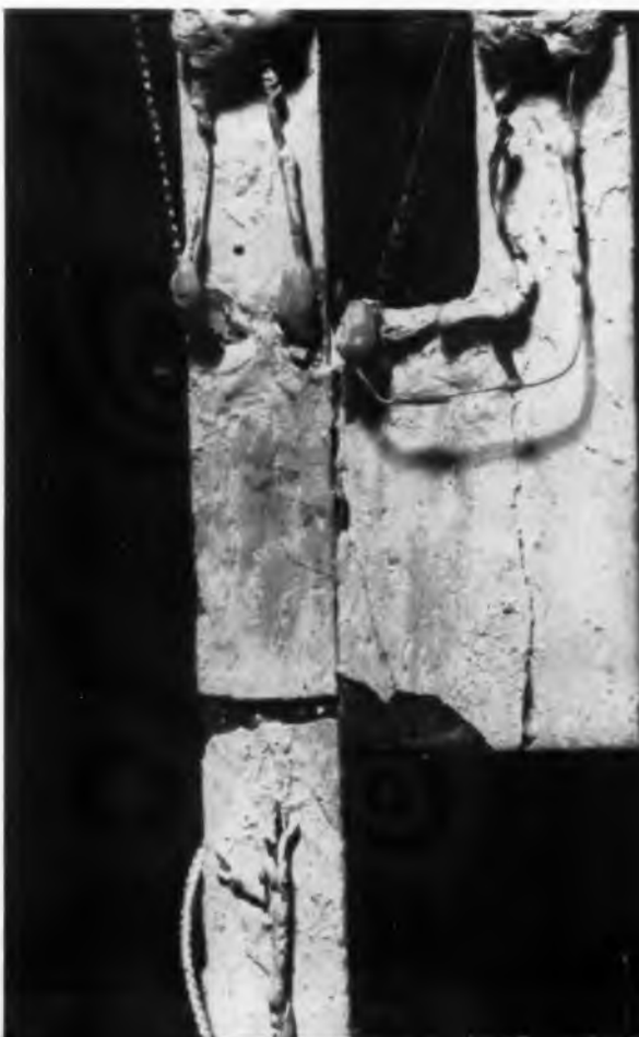
Fig. 3: Foil gage and ceramic cement installation after thermal shock. Foil and grid gages were limited by ceramic used to mount them.
