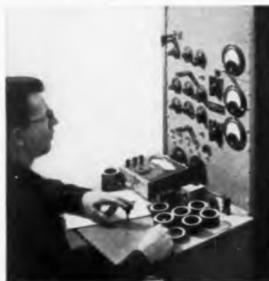
The Roberts Constant Current Flux Reset Method provides dependable core measurements.
