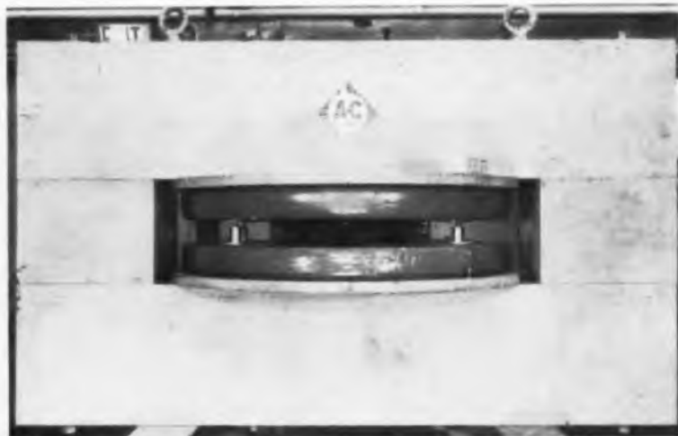
Fig. 2: Transistors, diodes, and tubes were tested in the field of this electromagnet
