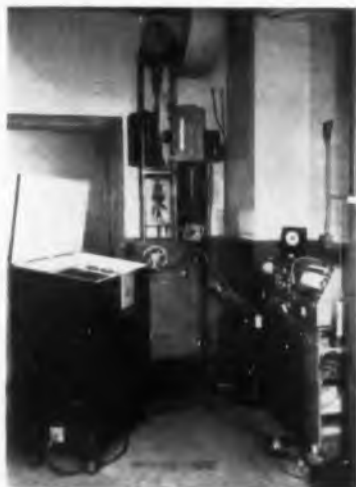
Fig. 2: "Dillon Dynamometer" adapted for elevated temperature testing, with controls and recording equipment. Note the radiant heat sources — two vertically mounted tungsten filament quartz tubes in air-cooled reflectors
