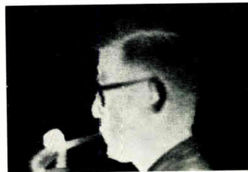
Fig. 5: Temperature drop through the stem of a pipe is shown by this I-R photograph.
