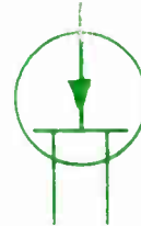
2. 5 P-type field-effects transistor.
