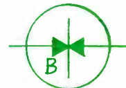
2. 20 Bipolar voltage limiter. (The arrowhead shall be of 60 degrees included angle; the point of the arrowhead shall touch the adjacent element symbol).
