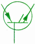
2. 7 P-N-P-N transistor (hook or conjugate-emitter connection).
