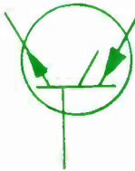
2. 8 N-P-N-P transistor (hook or conjugate-emitter connection).
