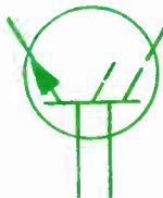
2. 17 N-P-I-P transistor with ohmic connection to the intrinsic region.
