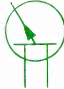
2. 4 N-type unijunction transistor (sometimes called double-base diode or filamentary transistor).
