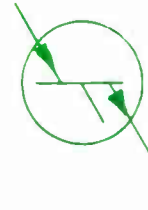
2. 11 P-N-P-N transistor without base connection.
