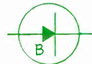
2. 19 Breakdown P-N diode. (The arrowhead shall be of 60 degrees included angle; the point of the arrowhead shall touch the adjacent element symbol).
