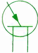
2. 3 P-type unijunction transistor (sometimes called double-base diode or filamentary transistor).
