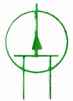
2. 6 N-type field-effects transistor.
