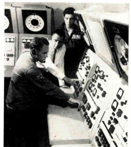
Air Force personnel simulate fueling of an Atlas ICBM missile at March AFB, Calif., as part of a human engineering study. Console of this type is used to prepare and fire missiles from a blockhouse.
