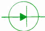
2. 18 P-N diode. (The arrowhead shall be of 60 degrees included angle; the point of the arrowhead shall touch the adjacent element symbol).
