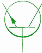
2. 2 N-P-N transistor (also N-P-I-N transistor, if omitting the intrinsic region will not result in ambiguity).
