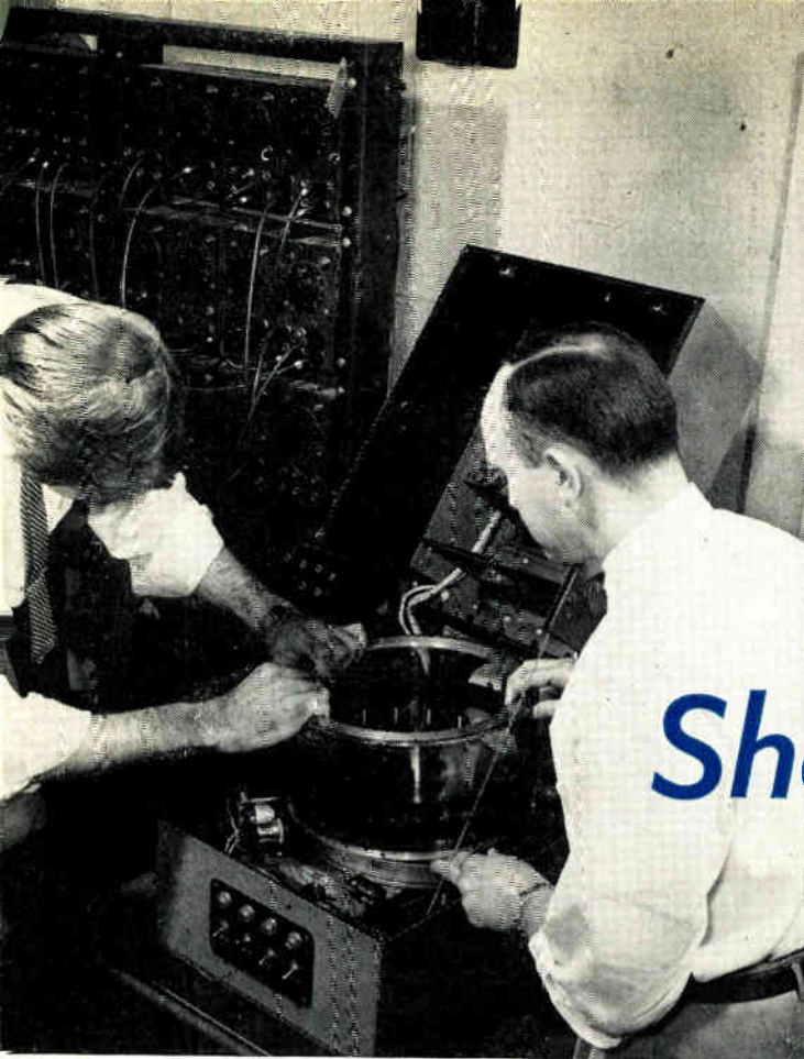
Fig. 1: A record of the aircraft's landing shock, traced on a transparent screen, is set on the drum of the function generator.
