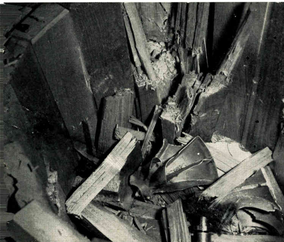
Fig. 1: The tremendous energy stored in the high speed rotor can be appreciated from this picture, which shows the destruction in the protective test chamber upon failure of the rotor.
