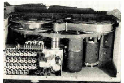
Fig. 2: The Tape Transport Unit contains the tape handling mechanism, a bias oscillator, mixing network, signal monitoring circuit, and remote control circuitry.
