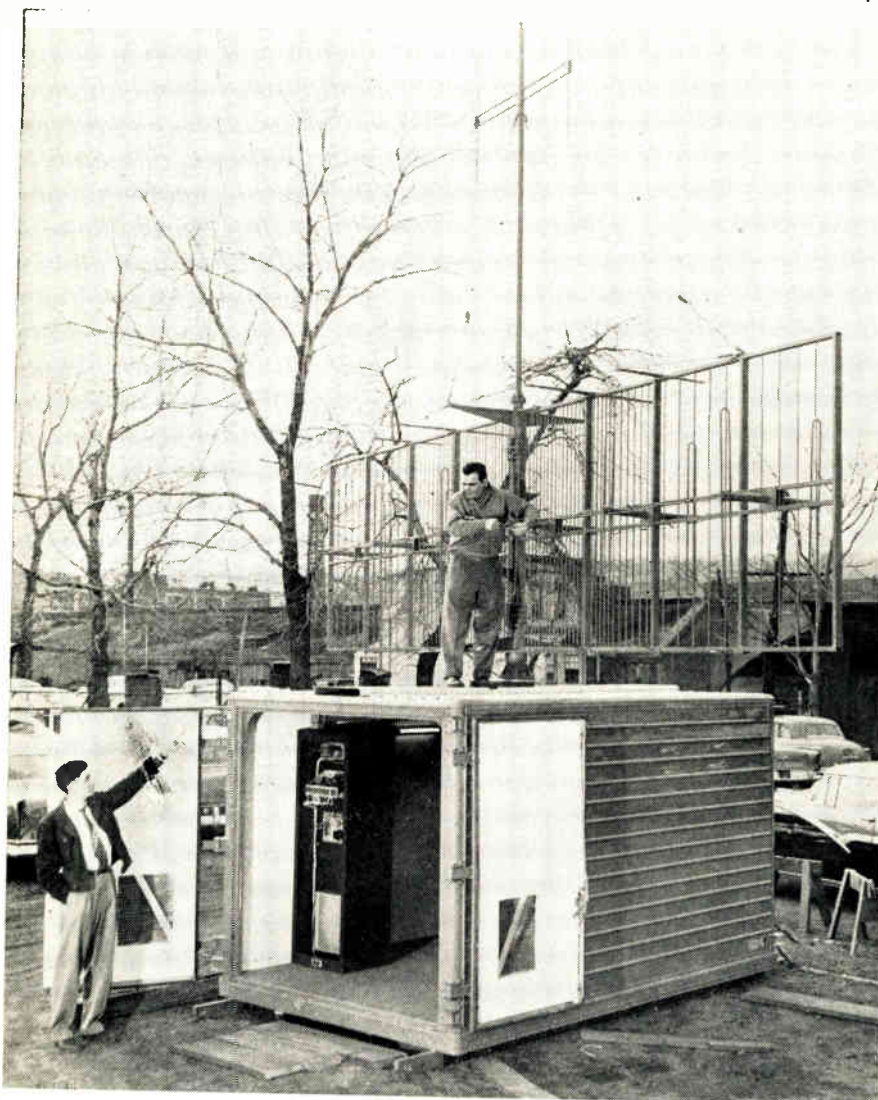
Fig. 1: The three antennas are mounted on the beacon body which rotates at two rpm.
