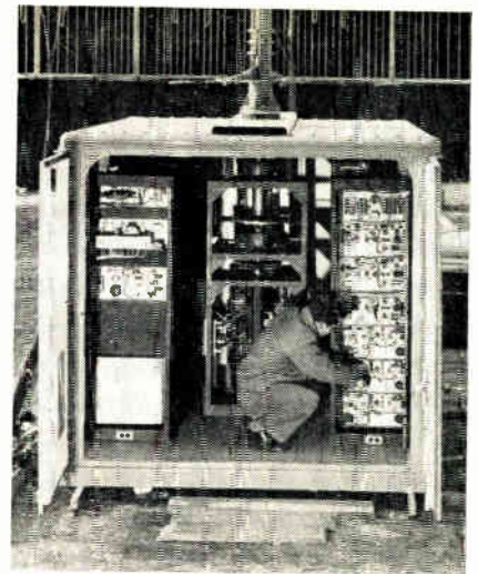
Fig. 2: The "Talking Beacon" is contained within a compact truck body; the antenna folds and stores within the body for transportation to a new location.
