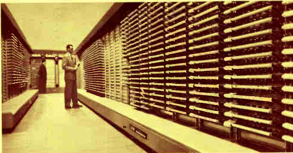
This huge computer, only a small part of which is illustrated, was engineered and built by IBM to serve as heart of the Semi-Automatic Ground Environment (SAGE) air defense system. G-E 5-Star 6414's in the computer had a perfect record of NO opens, shorts or mechanical defects.
