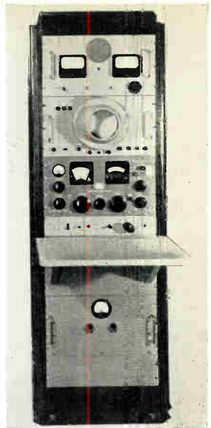
Fig. 11: Console, contains detector chassis, indicator, receiver and power supplies
