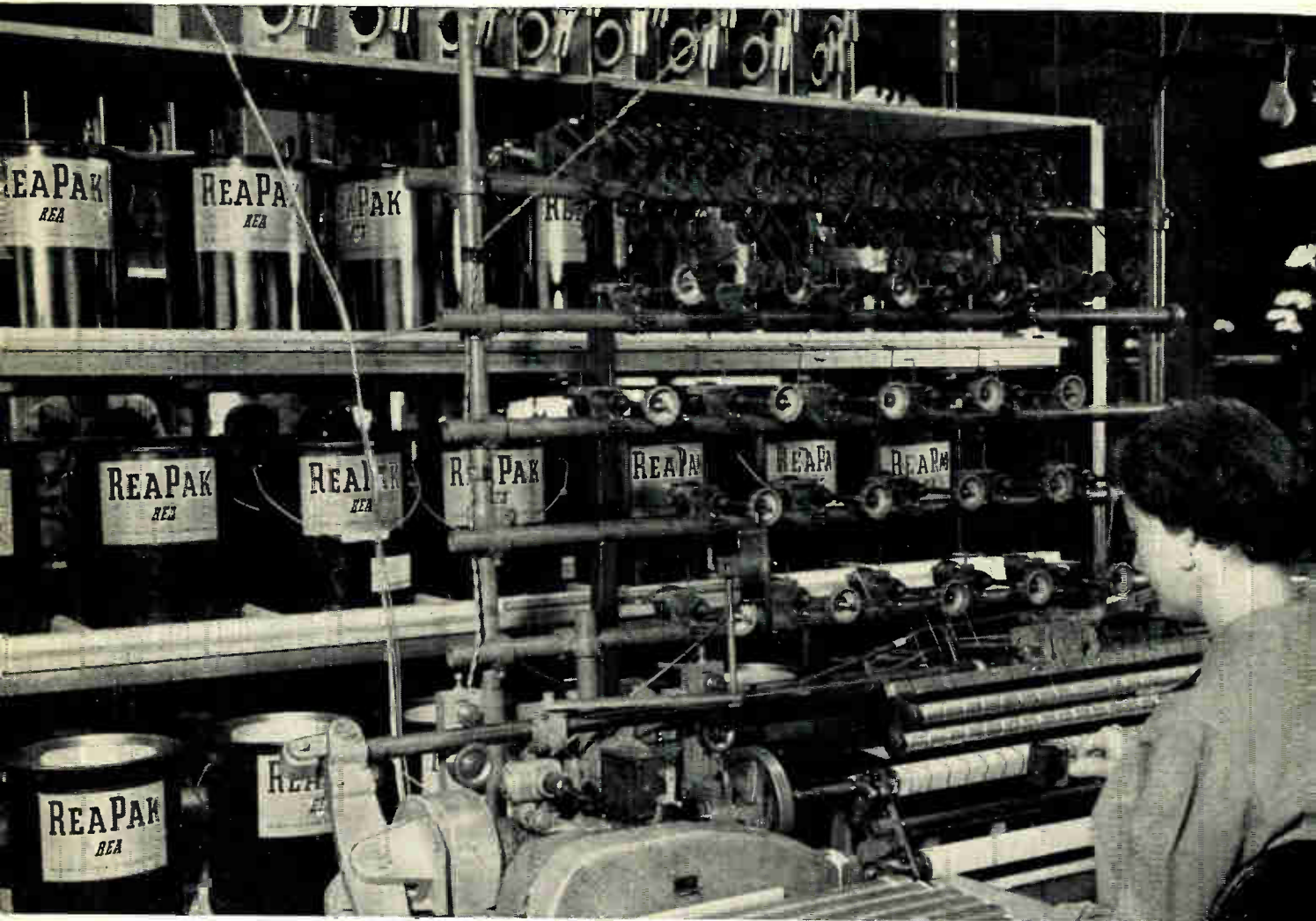
At Minneapolis-Honeywell, ReaPak Pails — holding 100 pounds of continuous length wire — replace the conventional spools holding only ten to fifteen pounds.
