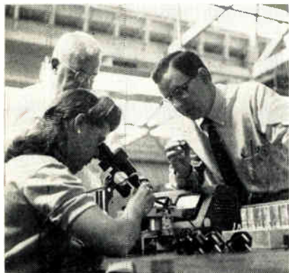
Fig. 2: Assembly of a precision potentiometer model requires use of a microscope.
