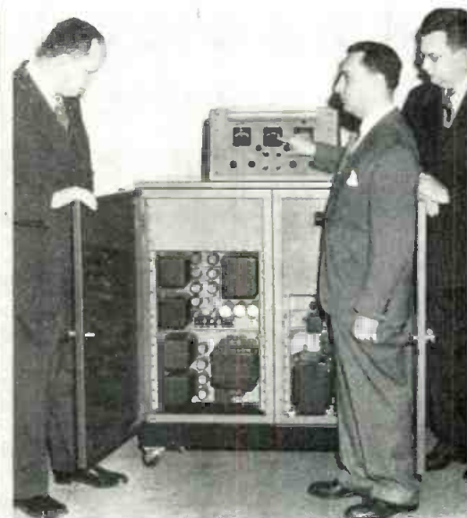
Fig. 2: (Left) RCA equipment using a 7-in. picture tube and a 20-in. spherical mirror to produce images 15 ft. x 20 ft. Fig. 3: (Right) Associated compact remote control unit incorporates control panel and plate power supply for projector. In typical installation this equipment may be installed within the regular film projection booth of the theater.
