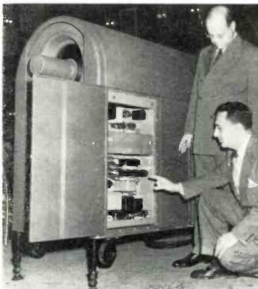
Fig. 2: (Left) RCA equipment using a 7-in. picture tube and a 20-in. spherical mirror to produce images 15 ft. x 20 ft. Fig. 3: (Right) Associated compact remote control unit incorporates control panel and plate power supply for projector. In typical installation this equipment may be installed within the regular film projection booth of the theater.
