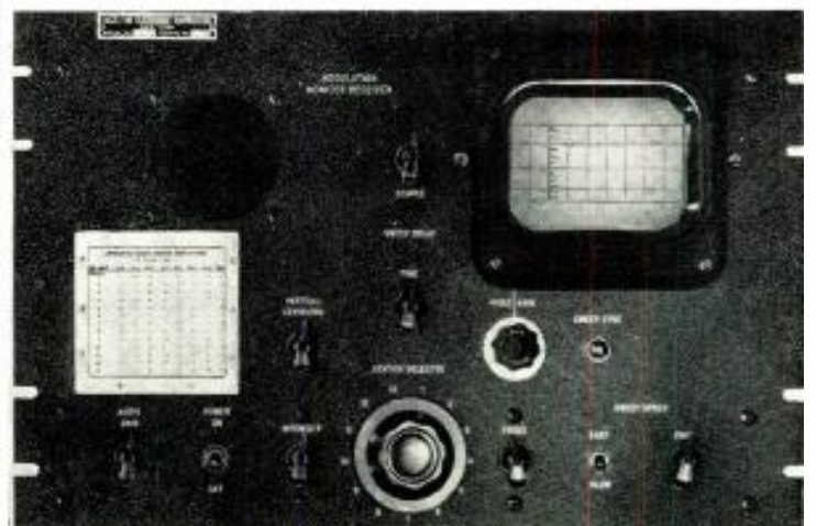
Fig. 3: (Below) Controls of model 1323, a modulation monitoring type receiver
