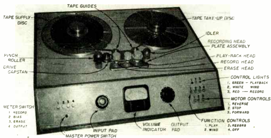
Fig. 1: (Above) Top view of the Model 100 Professional Tape Recorder identifies the various surface components and controls.
