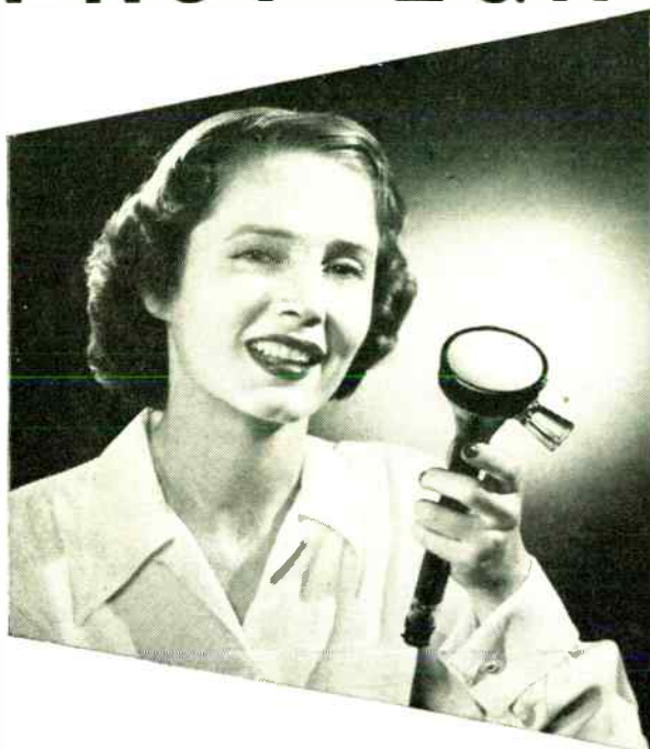
The 2½" magnetic projection triode 3NP4 has a face as small as a compact and is only 10½" long.
