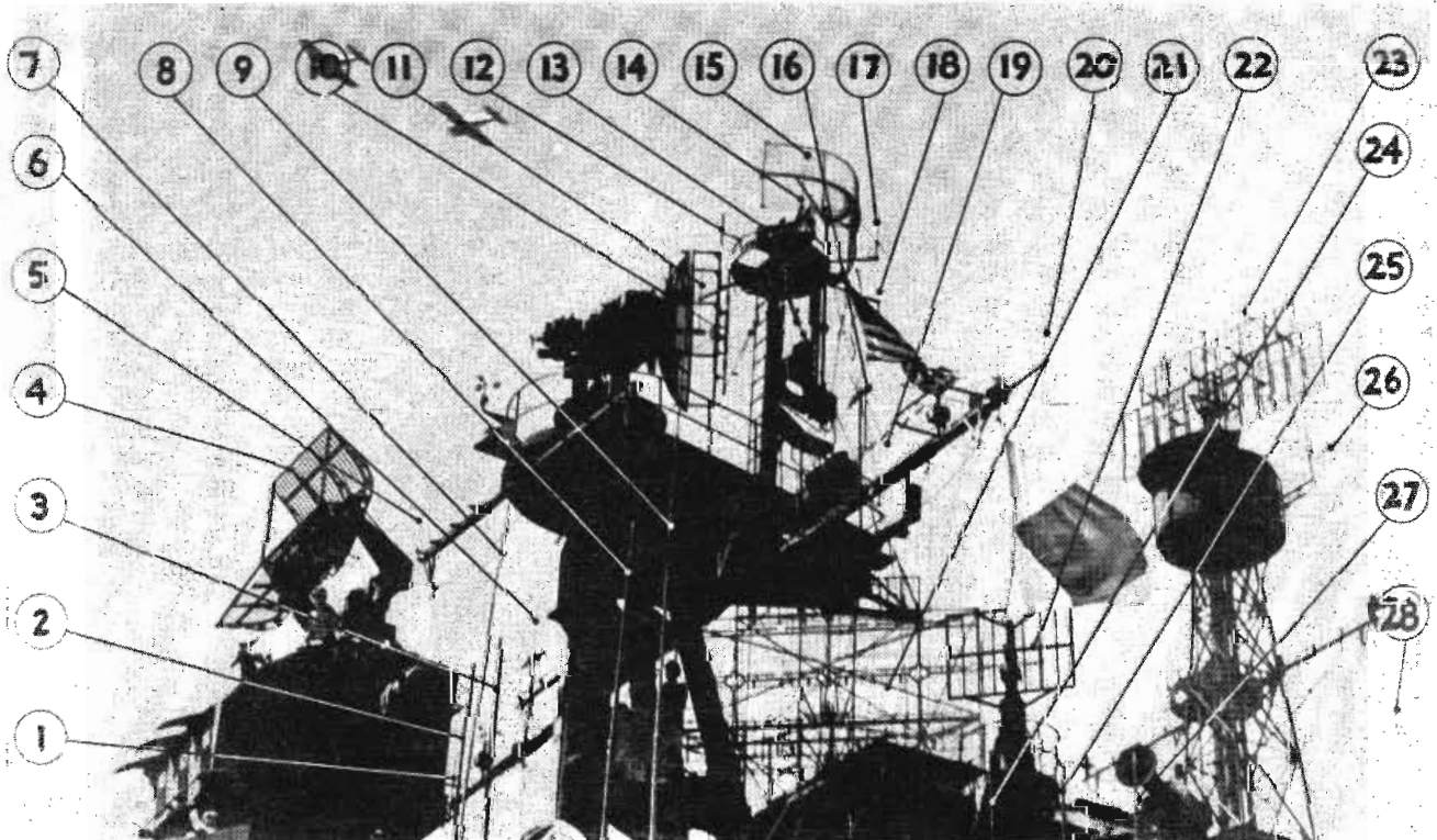
Looking up from the flight deck of the U. S. S. Lexington at the myriad radio-radar facilities, common to modern aircraft carriers. Antennas in this photo are used for the following purposes: 1, 2 and 3) radio communication; 4) fire control radar; 5, 6, 7, 8 and 9) radio communication; 10) air search and height finder radar; 11) radio communication; 12) radar test
