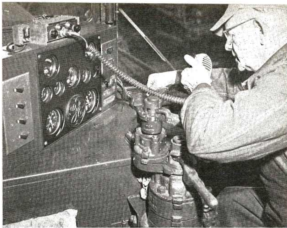
An engineer answers a call from the dispatcher in the Haskell & Barker industrial yard using Motorola equipment (a central station and six mobile units)
