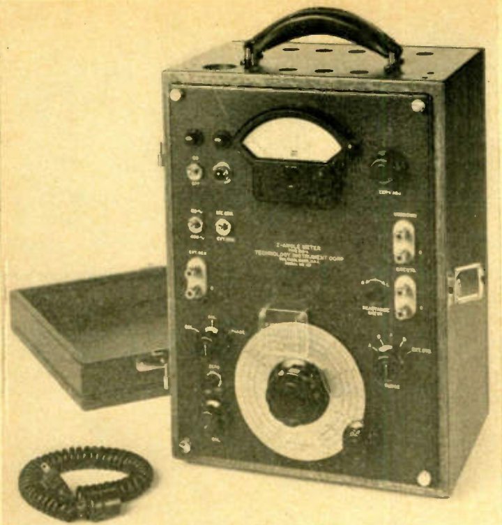
Fig. 1 — The type 310-A Z-Angle meter is self-contained in a small portable cabinet, including ac operated power supply, visual balancing and phase meter, impedance standards, and source for two common test frequencies
