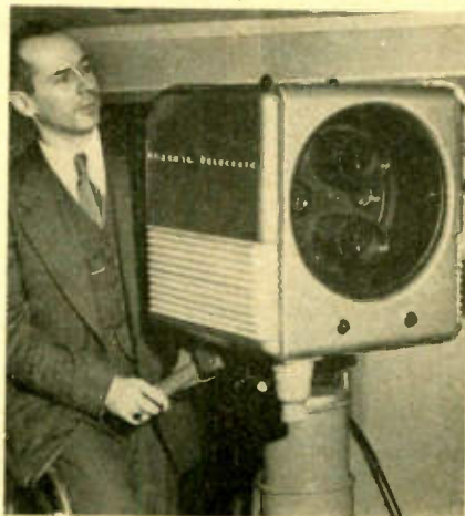
GE's new TV camera and one-man hydraulically operated dolly is lighter, more flexible in use
