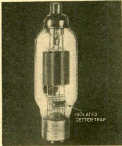
General appearance of tube showing location of the getter trap and its method of mounting
