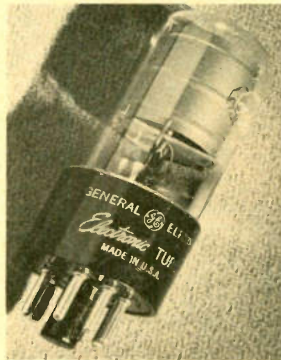
Fig. 1 (above)—Type 2B23 diode, showing standard intermediate-shell octal construction
