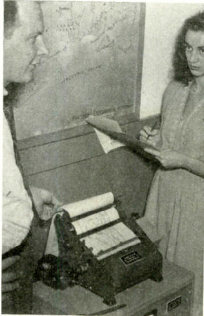
Raytheon's Waltham terminal with Hogan Fax receiver used in microwave demonstration
