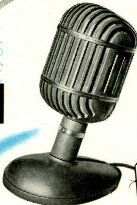
1937: The Western Electric "Machine Gun" mike does for sound pick-up what the telephoto lens does for photography. Sharply directional, this microphone makes sound "close-ups" at unusually long range.
