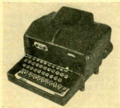
Code Typewriter directly converts letters into dots and dashes of any code system
