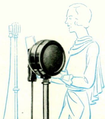
1931: Bell Telephone Laboratories developed the Western Electric moving coil or dynamic microphone. The first of its kind, it was rugged, noiseless, compact, and needed no polarizing energy. Many are still in use.
