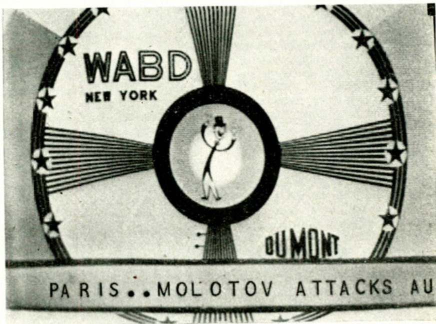
WABD, New York, in cooperation with International News, has found a way to make test patterns (transmitted by all TV stations at intervals to permit receiver adjustments) more interesting to the public, by adding superimposed news flashes. An enlarged projection of Teletype news tape (typed at about 60 WPM) is projected on a camera tube mosaic and fits into a space in the pattern designed for it, as above. Below, the Teletypewriter and reflection projector used in studio
