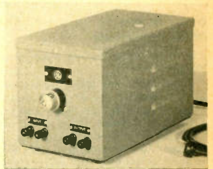
"Autopot" self-balancing potentiometer is a sensitive vacuum tube bridge circuit
