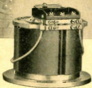
Seismometer assembly, showing magnet and bakelite bobbin at top.
