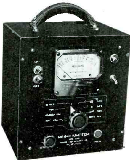
NO. 1020 MEGOhmmETER—a precision balanced electronic ohmmeter for the measurement of leakage resistance of insulating materials, condensers, cables, motor and transformer windings. The high voltage potential necessary for insulation measurements is included in the instrument. An exceptionally wide range of resistances can be measured on the six overlapping ranges, and is read directly on a 4" meter scale. A relay disconnects the high voltage from the binding posts to eliminate all danger of shock due to exposed high voltage potential.
