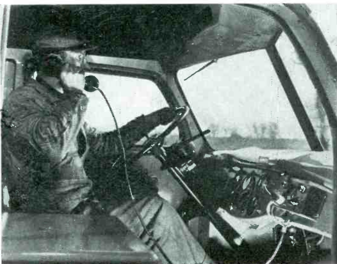
Two-way radio for trucks operates in the 156 to 162 mc band and uses FM
