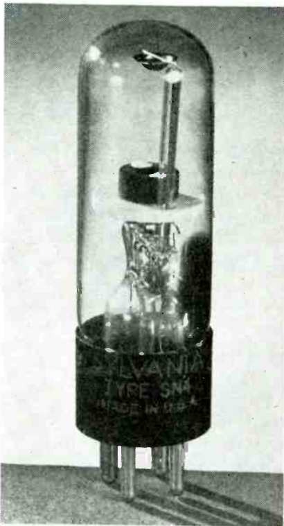
A light source for a stroboscope, the SN4 is an internally triggered, cold cathode, gas filled thyratron giving maximum illumination
