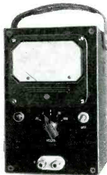
NO. 1030 LOW FREQUENCY "Q" METER—provides a frequency range from 50 to 50,000 cycles, with a range of "Q" measurements on coils from .5 to 500. The "Q" measurement may be made with as high as 50 volts across the coil with an accuracy within 5%. Tuning condenser range up to 11.11 mf. plus 1000 mmf. air variable. The stability and accuracy of measurement is unaffected by line variation.
