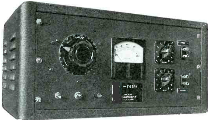
NO. 1050 60 CYCLE FILTER—for the calibration of instruments, where the form factor of the applied voltages is important (AC voltmeters and vacuum tube voltmeters), and for the measurement of harmonic distortion of amplifiers, transformers and tubes. The instrument is self-contained, AC operated, and is composed of a constant voltage transformer, a variac, a 60 cycle low pass filter, a decade attenuator, and a 1% AC voltmeter. The constant voltage transformer makes the instrument independent of the line variations. The variac makes the instrument extremely flexible and the decade attenuator makes it possible to vary the output voltage from 0 to 110 volts in increments of 1 volt.
