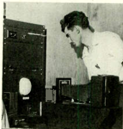
Method developed by Sylvania engineers for making photographic records of families of characteristic curves of various vacuum tubes
