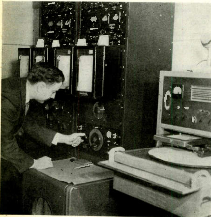
General view of one corner of one of the FCC monitoring stations showing arrangement of equipment used in monitoring and measuring
