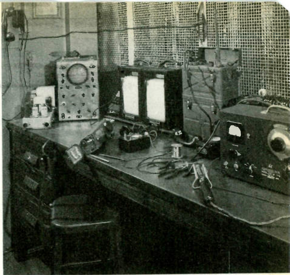
Repair and test section of the Pullman car electronic field laboratory of the Rock Island Railroad. From left to right there are illustrated an audio amplifier, a 5-in. oscillograph, a Mandi-talkie, a recording voltmeter and ammeter, a Walkie-talkie and a microvolter, beside the usual assortment of small tools and meters. The hanging phone (upper left) connects to the radios
