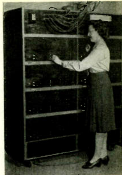
Fig. 14 Counter for aerodynamics range giving time in units of .625 microseconds to show slowing of bullet in its flight
