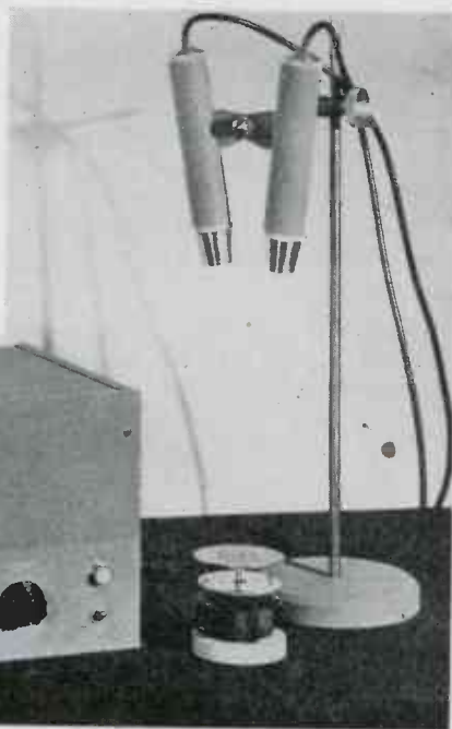
Method of setting up equipment for measurement of rotative speed in a horizontal plane
