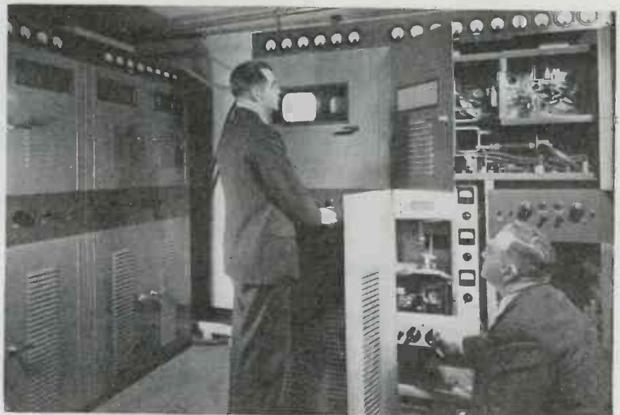
Early field tests are planned for this 300-mc television transmitter developed experimentally in RCA laboratories and still in the development stage. Engineers R. D. Kell and T. L. Gottier
