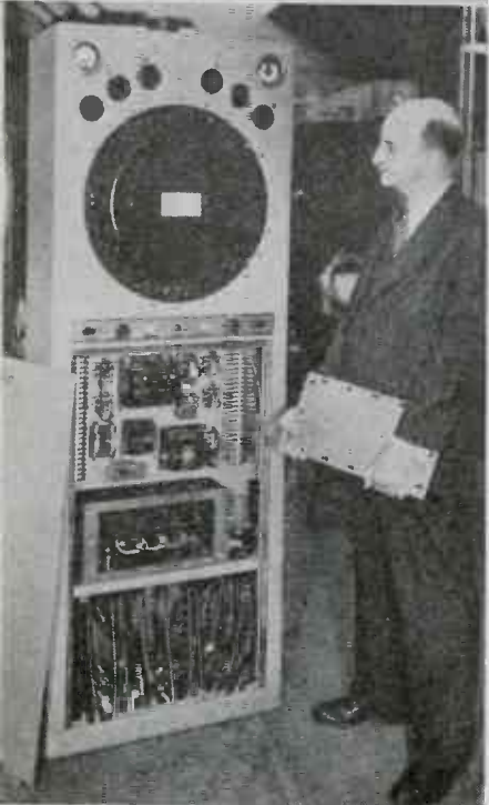
C. N. Cahusac, C-O-Two Fire Equipment Co., demonstrates the smoke detecting cabinet of the carbon dioxide shipboard fire extinguishing system. Heart of the unit is the photocell reflection detection method diagrammed below and described in the text
