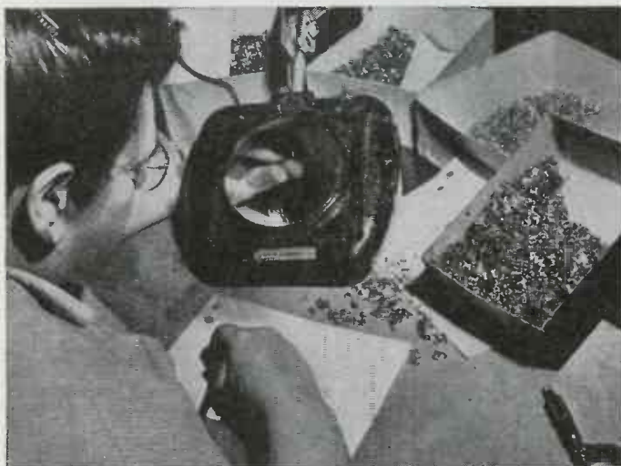
Tiny tube parts are magnified and their outlines superimposed on scale drawings to insure meeting the extremely close dimensional tolerances required.
