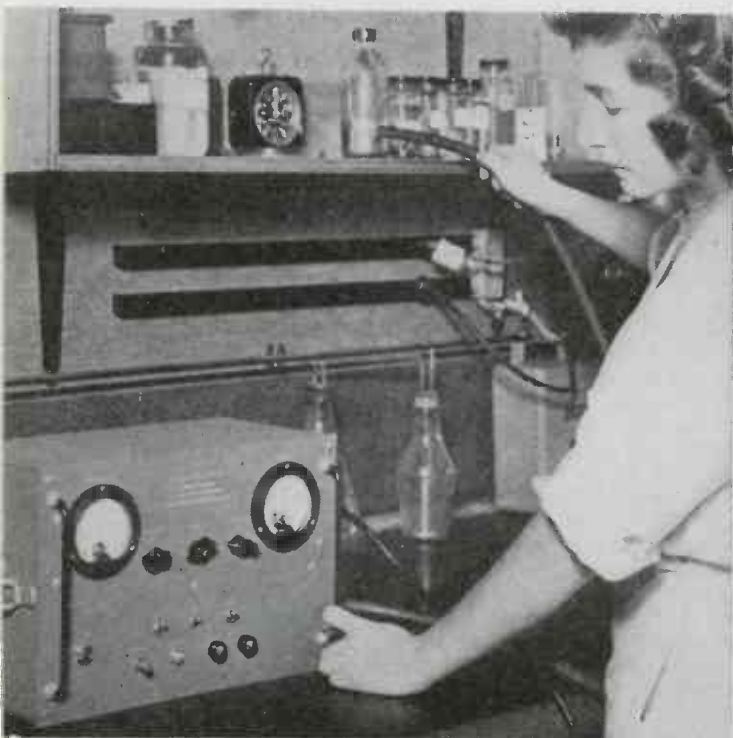
Sampling air at rate of half a cubic foot a minute, electronic detector measures mercury vapor concentrations of one part in 3,000,000 parts of air
