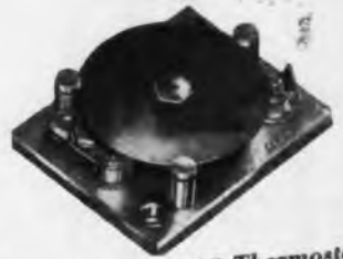
Type B-3120 Thermostat and Heater. Crystal Dew Point Control
