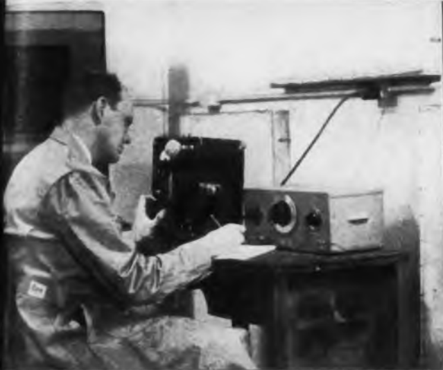
Sound intensity study. Photo shows sound level meter, audio oscillator and a loud speaker. The sound being measured is from "confidential" equipment close by but purposely not shown in this photograph
