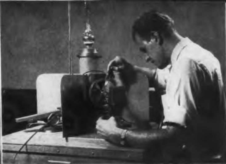
Metallurgical test using back-reflection X-ray diffraction technic. The four port XRD unit itself was constructed in the laboratories' shops, using a few stock parts and tube. Specimen is metal research product
