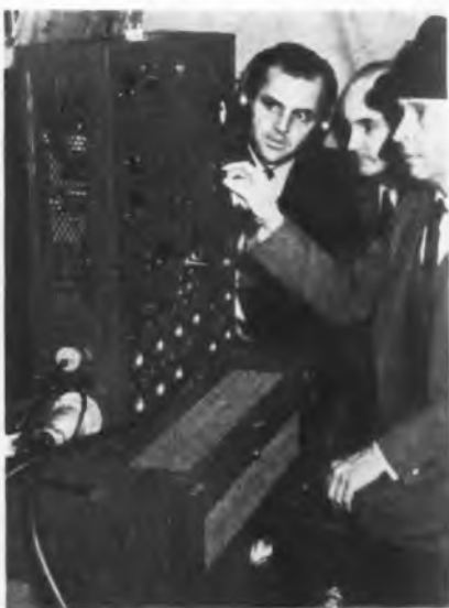
The 25-watt 324 mc transmitter used for televising sports and other local events
