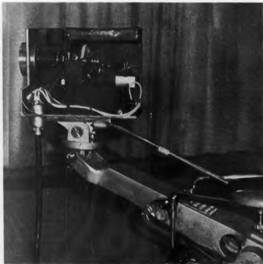
Construction of the iconoscope camera used 1937 to 1940 for live studio shows. Case below the iconoscope contains a preamplifier using three acorn pentode tubes
