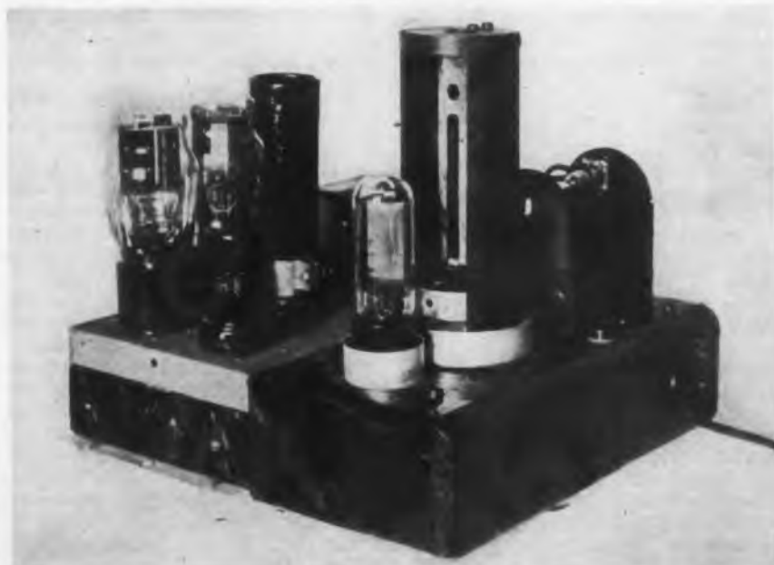
Fig. 4—Power supply unit showing 1,000-cycle tuning fork, lamp lenses, photoelectric cell, amplifier, and driving magnet. Form-fitting covers normally enclose the fork and optical system
