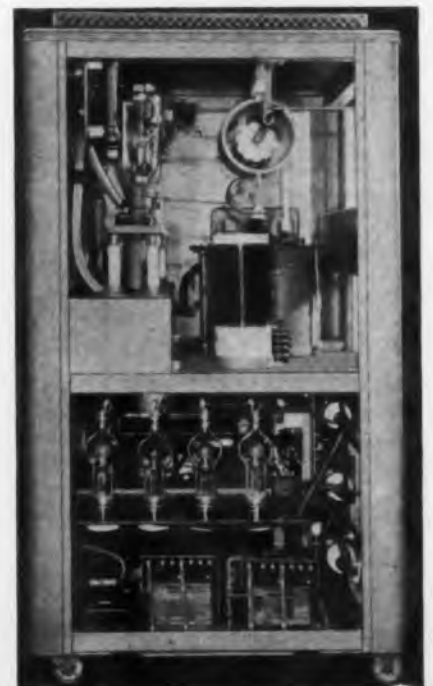
Fig. 3. Twenty kw power oscillator using city water to cool tubes, plate tank, and work coils
