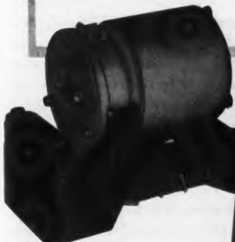
Leland Carbon Pile Voltage Regulator—control device on air-borne electronic equipment component.
