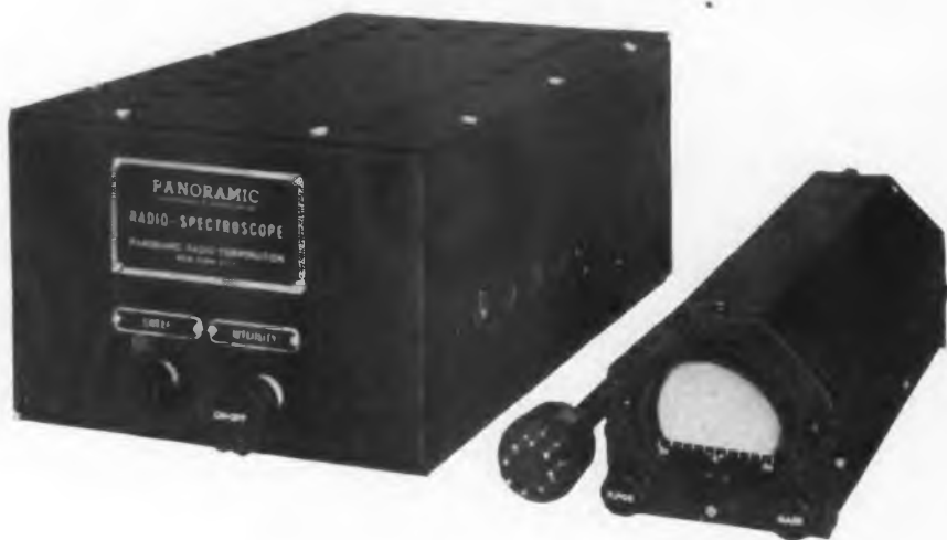
Fig. 6—One model of adapter designed for mobile installation uses 2-inch CRT in separate case
