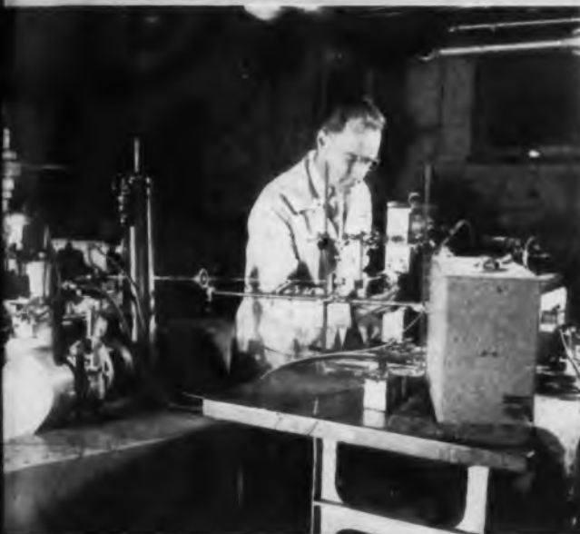
Diesel engine study, using Edgerton high speed motion picture camera to photograph combustion through special port. Many electronic aids for engine analysis are used in Armour's internal combustion research
