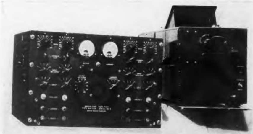
Fig. 2—One of several four-channel amplifiers with multi-channel oscillograph used by CAA in measuring and recording resonant vibration frequencies that cause fatigue
