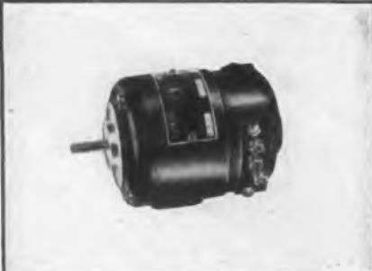
Type "B" A.C. Generator Permanent Magnet Field wound for one, two or three phase A.C. Ball-bearing equipped; flange or base mounted. 2 1/4" outside diameter . . . weighs 16 ounces.
