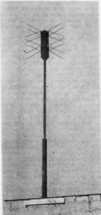
The 324 mc beam relay receiving antenna has 16 half wave elements in four groups
