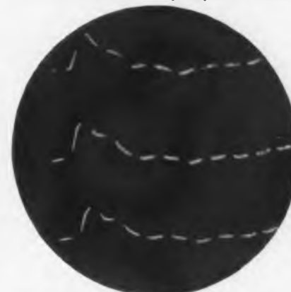
Fig. 6—Shows the use of modulated cathode ray beam for timing purposes. Three repeated readings are shown here
