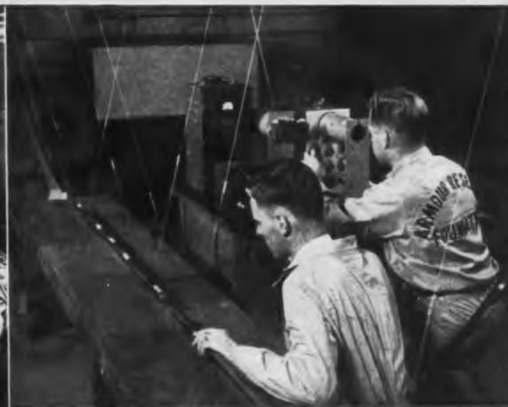
Calibrating strain gages, using bridge, amplifiers, oscillograph, and camera. Strain gages are fixed to one suspended metal bar, struck with known force by other bar in foreground as gage's response is recorded
