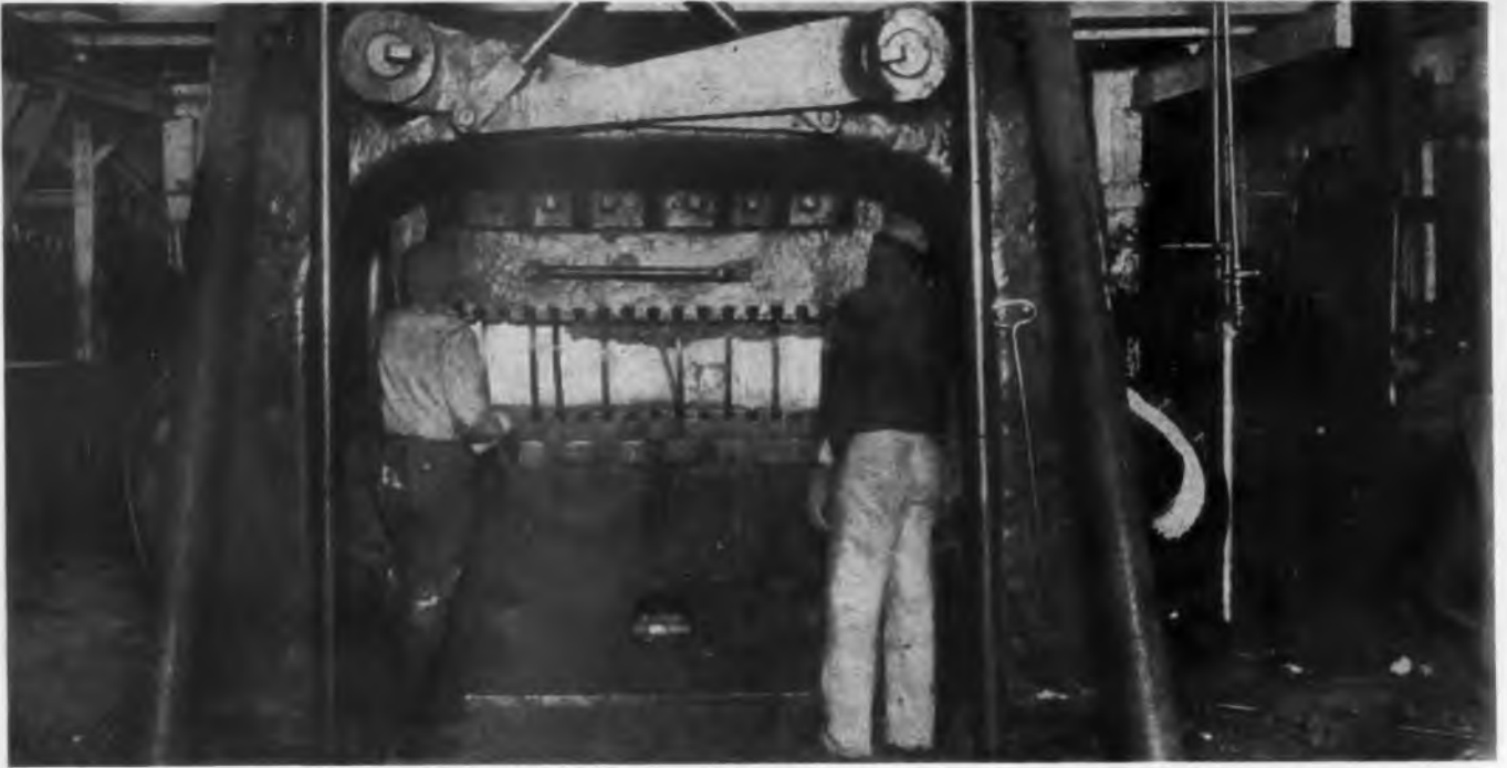
Fig. 1—Compress for compressing cotton for shipment. Densities as high as 35 lbs./cu. ft. are produced equal to that of the heaviest pine lumber
