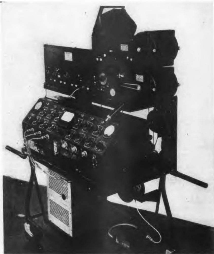
Fig. 5—Cotton pressure recorder complete with chassis. The control and reading unit stands on the main table, with the power supply underneath, and the oscillograph on the shelf at the top. Provision is made for winding the leads to the measuring elements so that all of the instruments remain properly connected during transportation. One pressure element in V-block on lower shelf
