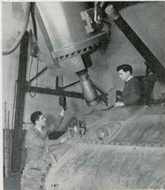
INSULATED WITH compressed gas instead of oil, which permits reduction of its bulk by two-thirds, this million-volt General Electric X-ray machine is used by the Ford Motor Co. for inspecting welds in the armor-plate skin of M-4 tanks and M-10 tank destroyers hulling in Detroit factories
