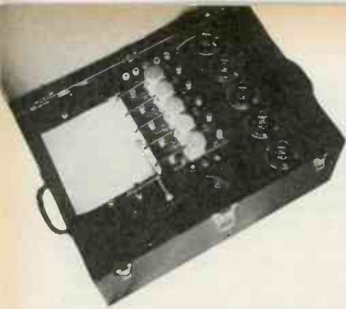
FIVE CHANNEL direct writing oscillograph, the Garceau Velograph
