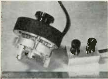
Fig. 5—Resistors in 18C attenuator are virtually buried in aluminum block to avoid undesirable coupling
