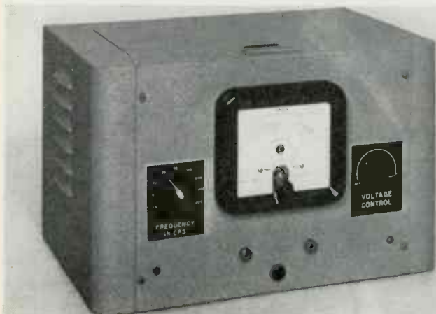
CORTICAL STIMULATOR , used in nerve and mental therapy, delivers an electrical shock of prescribed strength. Rahm Instruments, Inc.
