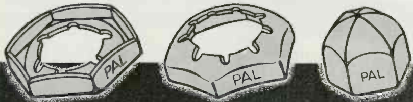
DOUBLE LOCKING ACTION When the PALNUT is wrench-tightened, its arched, slotted jaws grip the bolt like a chuck (B-B) while spring tension is exerted upward on the bolt thread and downward on the part (A-A), securely locking both.
