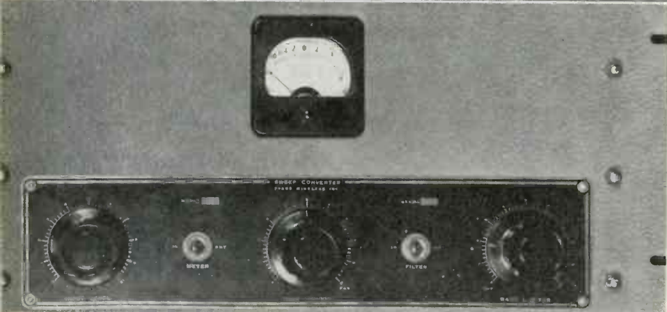
TRANSMITTING STATION INTERIOR (left above), showing a portion of the 26 transmitters and the antenna patching system. Right, the 40 kw telegraph-telephone transmitter. Left, sweep converter panel of the new style anti-fade equipment
