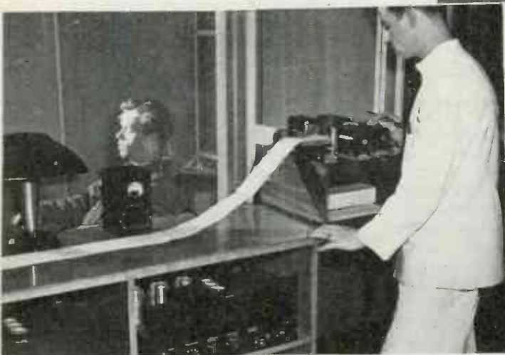
GRASS ELECTROENCEPHALOGRAPH —Used for brain wave analysis with 4-pen recorder
