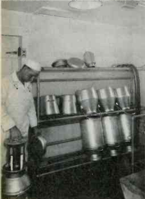
DESTROYING SURFACE BACTERIA by irradiating insides of milk cans with 2537 Angstrom unit ultra-violet. Additional Sterillamps on ceiling
