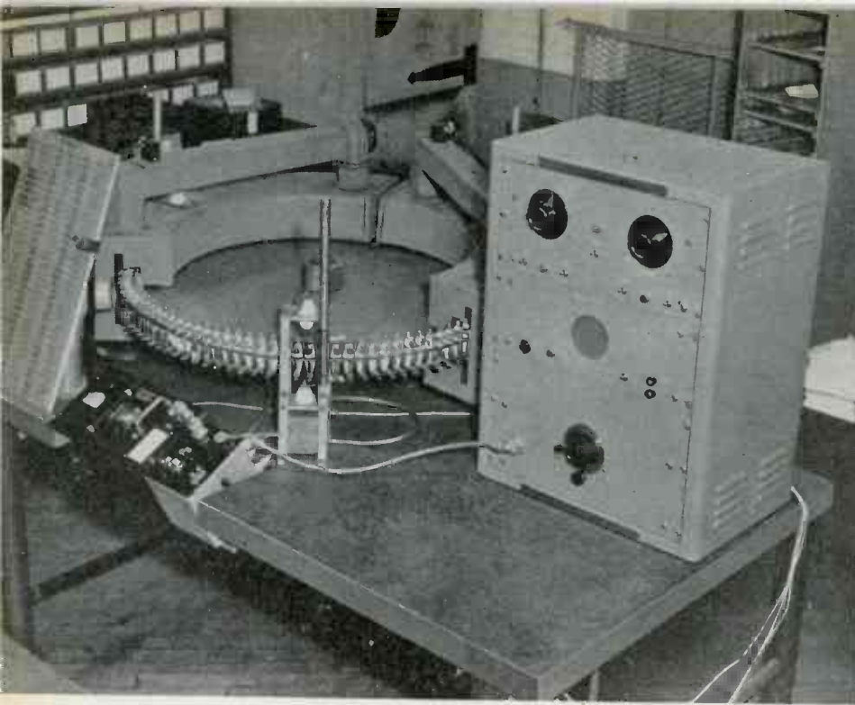
TEST APPARATUS , designed by Erie Resistor engineers, permits individual tests on the temperature coefficient of Ceramicons, at 25 deg. C. to 85 deg. C.
