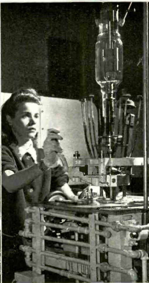
↑ TUBE-SEALING speed was doubled by switch from horizontal lathe to vertical outfit which holds tube stationary while torch cluster revolves, at Westinghouse Lamp Division
