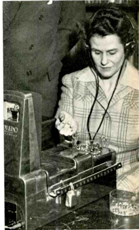
Blind girl is able to weigh accurately by listening for continuous tone
