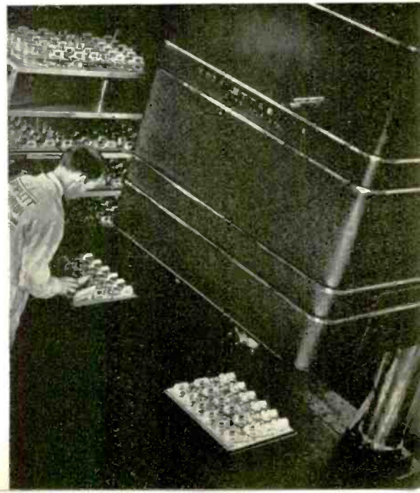
Electronically timed controlled high-speed X-ray for small parts inspection
